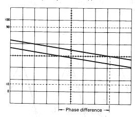
Expanded sweep waveform display.
