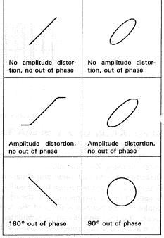
Fig. 17 Typical phase measurement oscilloscope displays
