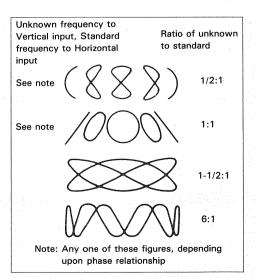
Fig. 48 Lissajous waveforms used for frequency measurement
