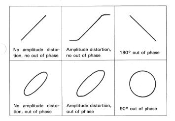
Fig. 47 Typical phase measurement oscilloscope display
