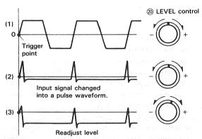
(a) When the trigger level is set around the center of the waveform.
