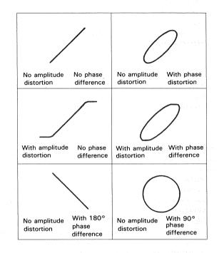
Fig. 51 Typical Display of Phase Measurement
