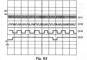
Example of simultaneous display of main sweep and delayed sweep (at  $\times$  10 magnification) Setting of controls
