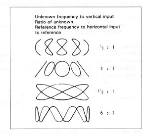
Fig. 52 Lissajous' Pattern used for Frequency Measurement
