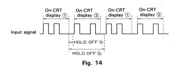
If the HOLDOFF is set like a , waveforms (1) and (2) are displayed on the CRT alternately.
