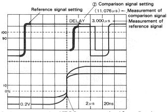
Read measurements when AFT.D  $\dot{\textbf{B}}$  sweep traces 1 and 2 are adjusted to same position
