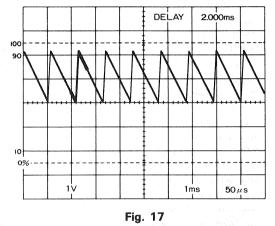
By setting the HORIZONTAL MODE switches to ALT, c) two trace lines of the A sweep and B sweep are displayed alternately, enabling magnified and nonmagnified parts to be observed simultaneously. If trace lines of the A sweep and B sweep are hard to be observed due to overlapping, control the TRACE SEP ③ to shift the B sweep waveform to an easyto-see position.
