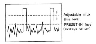
Figure 6. Example trigger level adjustment
