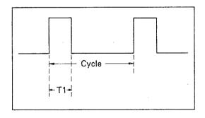
Figure 5 Duty cycle measurement
