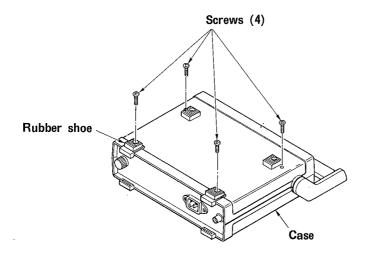
Fig. 5 Disassembly and Assembly of Case
