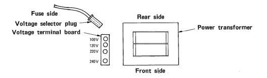
Fig. 6 Internal Selection of Supply Voltage
