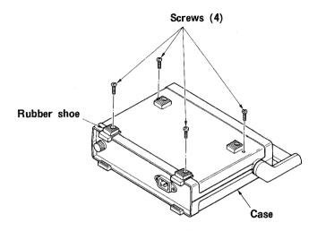
Fig. 5 Disassembly and Assembly of Case
