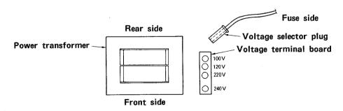
Fig. 6 Internal selection of Supply Voltage
