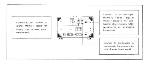
Fig. 5 Out put terminal on rear panel
