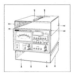
Fig. 7 Removing the case
