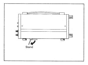
Fig. 2 Use of auxiliary foot
