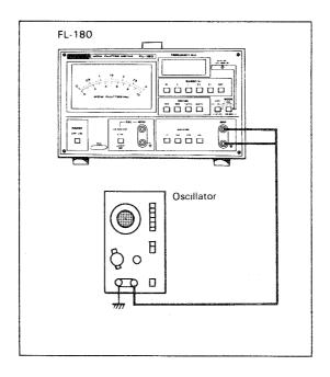
Fig. 6 Connection of the FL-180 and the oscillator
