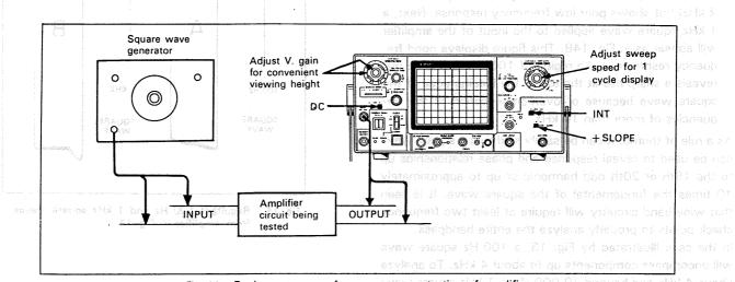
Fig. 11. Equipment set-up for square wave testing of amplifiers COO. Of provide boot sHX & evolu-
