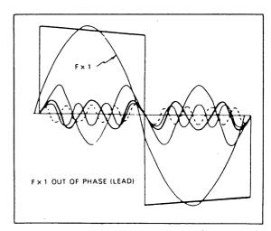
Fig. 17. Tilt resulting from phase shift of fundamental frequency in a leading direction
