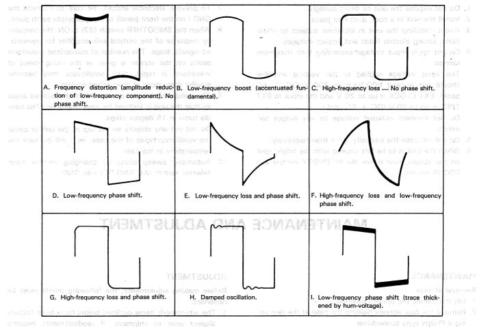
epstion storage is wood Fig. 22.11 Summary of waveform analysis for square wave testing amplifiers u and box learning as and usual. Fig. 22.11 Summary of waveform analysis for square wave testing amplifiers u and box learning as a storage of the storage of the
