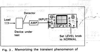
mechanical impact waveforms
