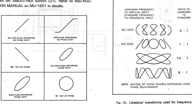
Fig. 8. Typicl phase measurement oscilloscope displays
