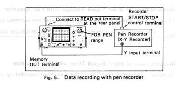
To record memory data with pen recorder (X-Y recorder), make connection as shown in Fig. 7 and operate the scope as follows:
