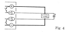
If the load is too far apart, oscillation may be caused by the output line inductance and capacitance. In this case, connect an approximately 100  $\mu$ F electrolytic capacitor in parallel with the load terminal.
