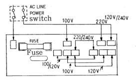
Voltage switching and fuse P.C board
