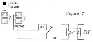
OUTPUT terminal closed : Output off OUTPUT terminal opened : Output on Set the OUTPUT switch on the panel to ON for operation.
