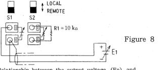
Relationship between the output voltage (Eo) and external voltage (E1)
