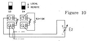
Relationship between the output current (I<sub>0</sub>) and external voltage(E2)  $I_{0} = \frac{I_{max}}{10} \times E2 \text{ (A) } I_{0}: \text{ Output current} \\ (0 \leq E2 \leq 10 \text{ V}) \\ E2: \text{ External voltage}$
