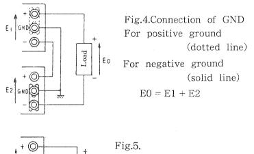
+E: Intermediate point is hooked up to ground.
