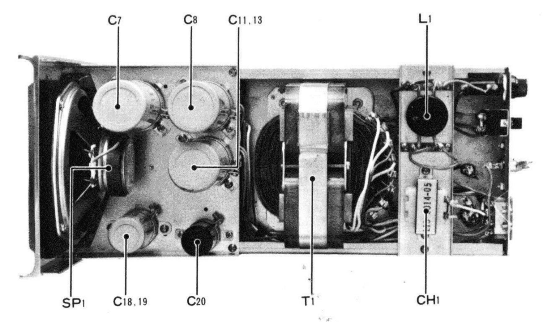
FIGURE 3. Top Chassis Parts Diagram.
