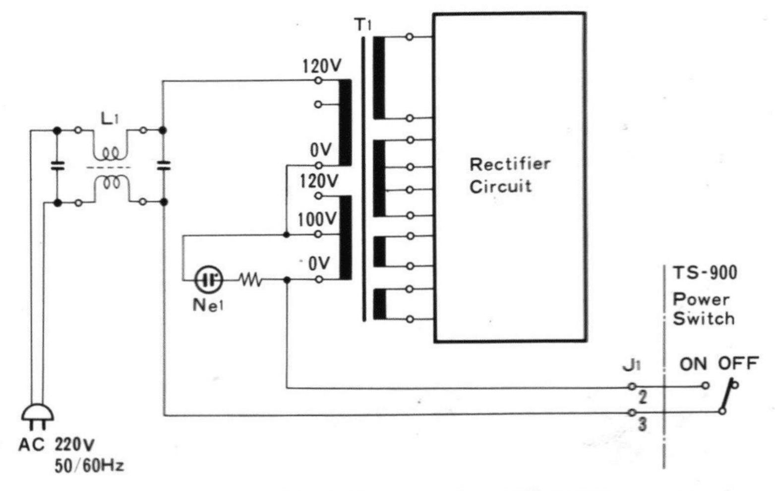
FIGURE 5. Block Diagram (on 220 VAC operation)
