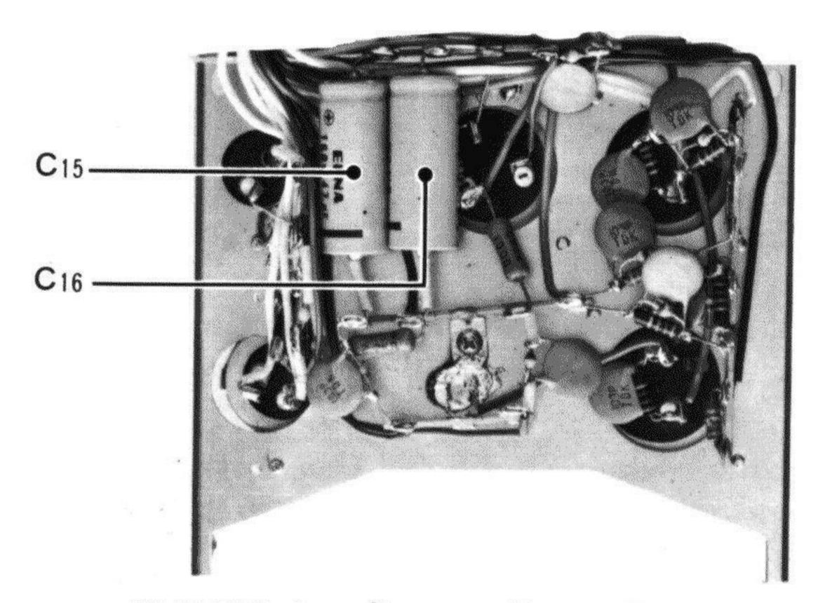
FIGURE 4. Bottom Chassis Parts Diagram.
