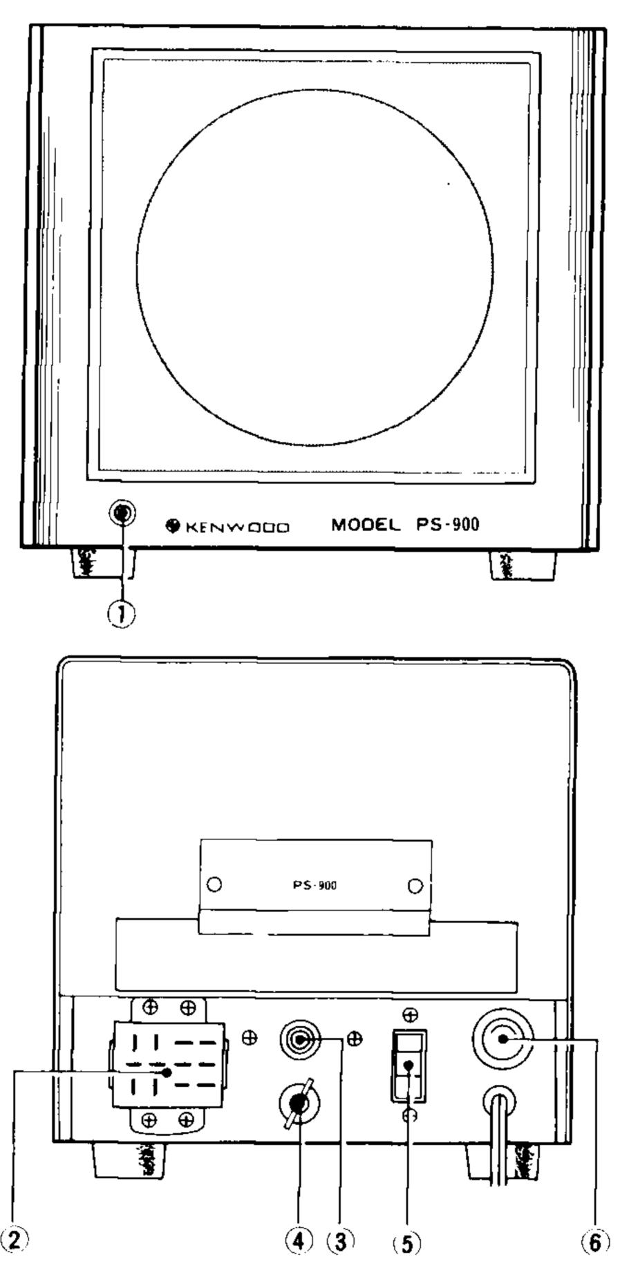
FIGURE 2. PS-900 Operating Controls
