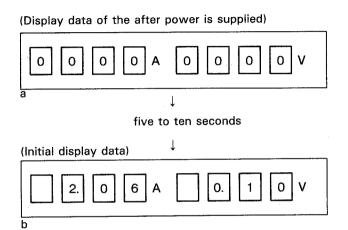
\* The display panel of the PWR36-1 indicates the two values: 1.04 A and 0.10 V.
