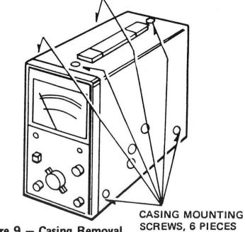
Figure 9 — Casing Removal.
