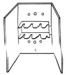
Figure 10 - PC Board Retainer.
