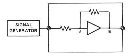
Figure 8 - Negative Feedback Amplifier Gain Measurement.
