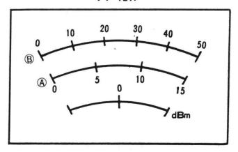
Figure 5 — Meter Scale Graduations.
