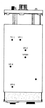
Fig. 5 Input Unit Adjust: ts (Bottom View)
