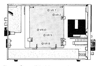
Fig. 6 Output Unit Adjustments (Left Side View)
