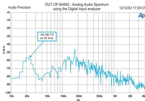
Figure 8 Spectrum analysis of the noise output of an over-sampling D to A converter showing large noise signals above 20 kHz and well out to 4 MHz.
