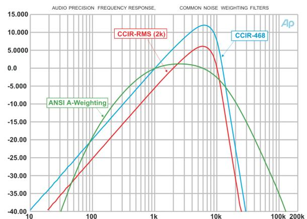
Figure 7 Common Noise Weighting Curves: ANSI/IEC “A-Weighting, CCIR-468, and CCIR-RMS.
