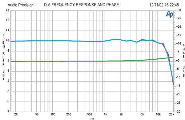
Figure 6 Typical Frequency and Phase Response
