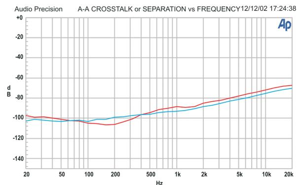
Figure 11 Interchannel crosstalk: left into right, right into left.
