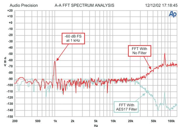
Figure 9 Spectrum analysis of an over-sampling D to A converter with and without the use of an AES17 filter.
