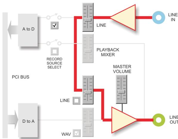
Figure 5b Analog loop-through path (mixer) - Line In to Line Out
