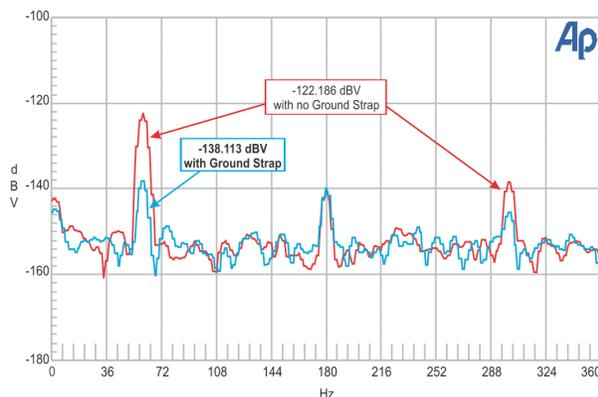
Figure 4 Spectrum analysis of noise with and without supplementary ground connection showing increase in mains hum level.
