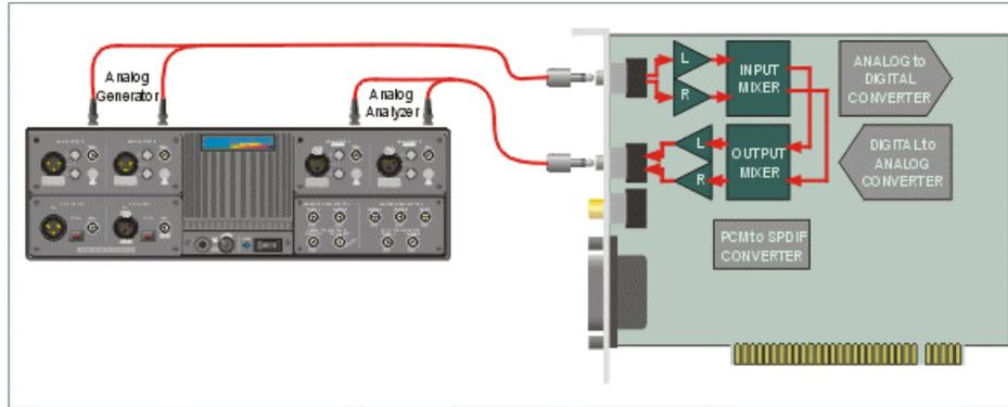
Signal source is Audio Generator to Line Input
