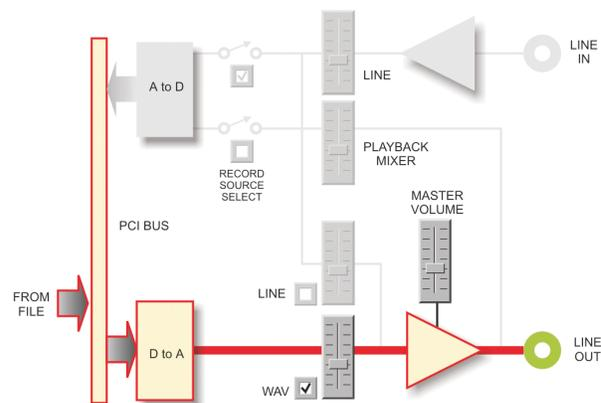
Figure 5 a PC to DA Playback Path
