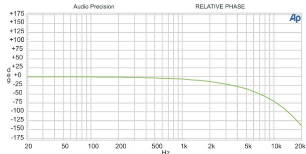
Figure 10 Phase response of a audio device with a one-sample offset of the second channel.
