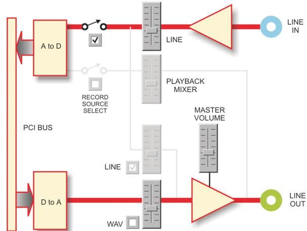
Figure 5d AD to PC to DA (Record-Play Converter loop) Path
