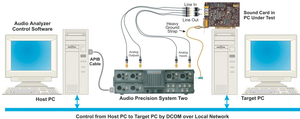
Figure 3 Test Setup. The host computer runs the test software and controls the audio analyzer. The target computer contains the PC audio device and runs a small control application that allows it to communicate with the host computer.
