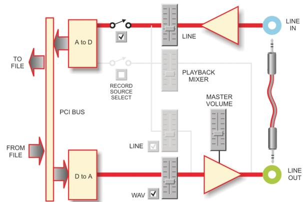
Figure 5e PC to DA to AD to PC (Record/Play loop) Path
