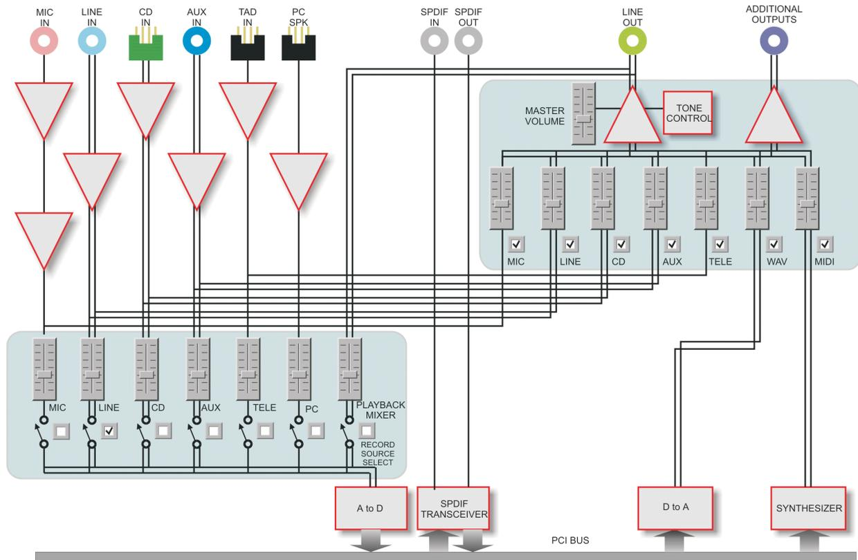
Figure 1 Block diagram of a typical PC audio device
