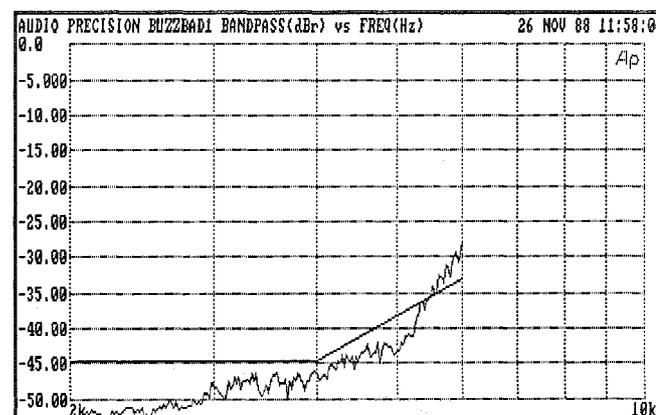
**Figure 25 Rub and Buzz Test Result, Bad Tweeter #1**
