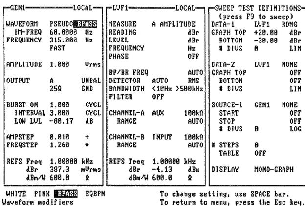
Figure 13 Setup Panels, Sensitivity Test Using 1/3 Octave Pink Noise
