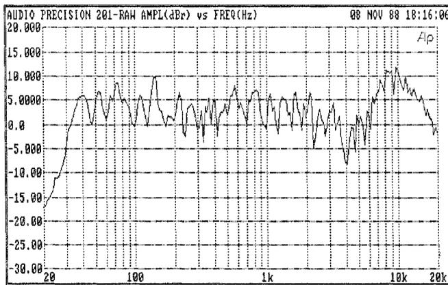
Figure 4 201-Point Measurement, Full-Range Speaker System in Reflective Space
