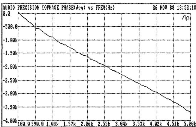
Figure 19 Input-Output Phase, Loudspeaker to Measurement Microphone
