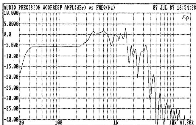
Figure 2 Anechoic Chamber Full-Spectrum Measurement of 15-Inch Woofer in Baffle
