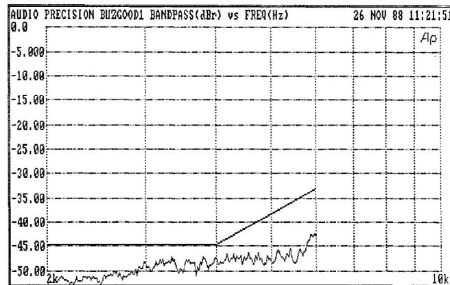
**Figure 23 Rub and Buzz Test Result, Good Tweeter #1**
