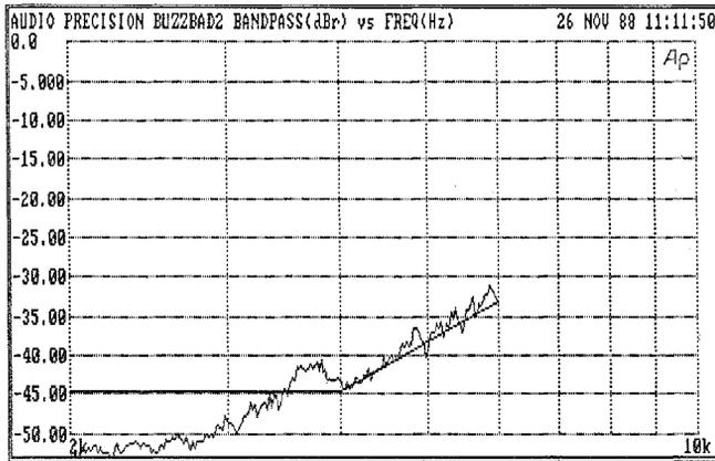
Figure 26 Rub and Buzz Test Result, Bad Tweeter #2
