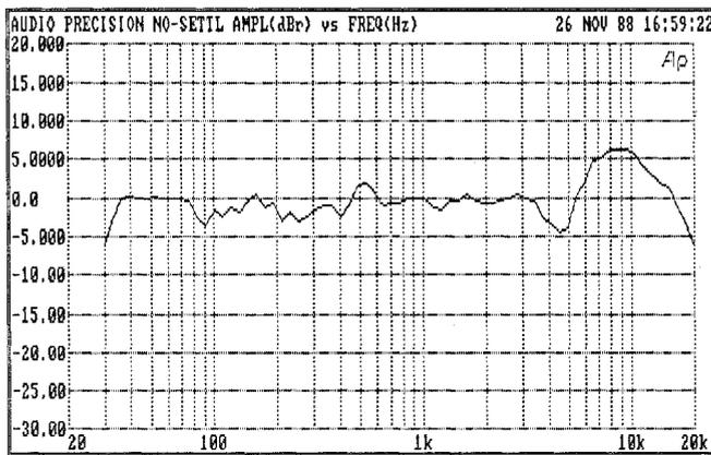
**Figure 12** Response Graph (After Smoothing), NO-SETTL.TST for Faster Testing
