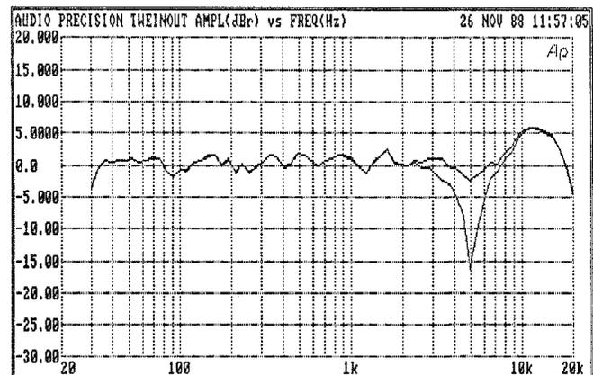
Figure 14 Superimposed Graphs, Tweeter in Correct and Incorrect Polarity
