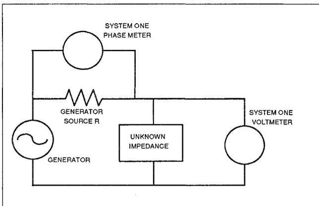
Figure 30 Simplified Equivalent Circuit, Impedance Tests
