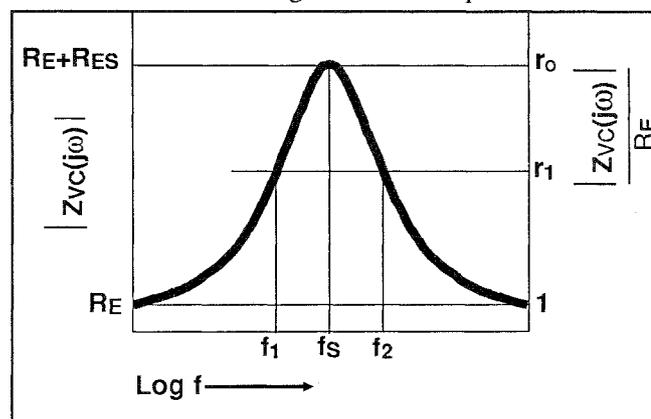
Figure 3 Driver Voice-Coil Impedance Magnitude
