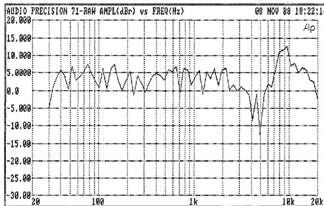
Figure 5 71-Point Measurement, Full-Range Speaker System in Reflective Space
