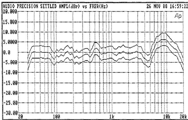
Figure 9 Data With Smoothed Upper and Lower Acceptance Limits, Offset  $\pm 3$  dB
