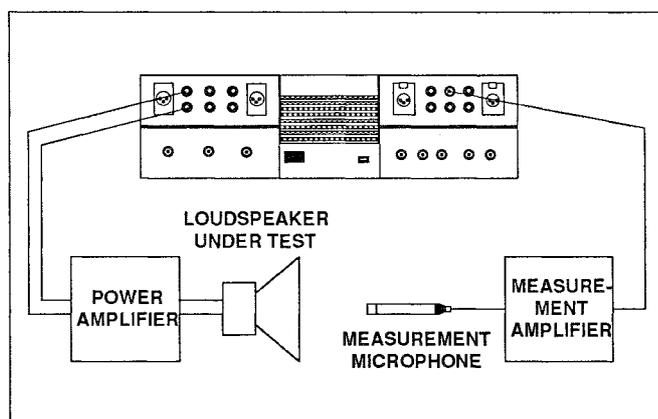
**Figure 1** Hookup Diagram for Response, Sensitivity, Polarity, and Rub and Buzz Tests
