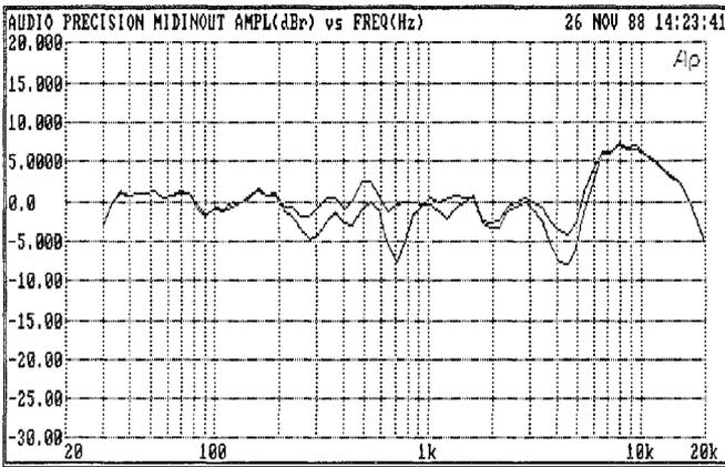
Figure 15 Superimposed Graphs, Mid-range Driver in Correct and Reversed Polarity
