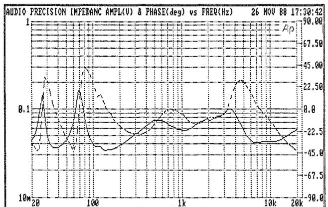
Figure 28 Magnitude and Phase of Impedance vs Frequency, Four-Way Loudspeaker System
