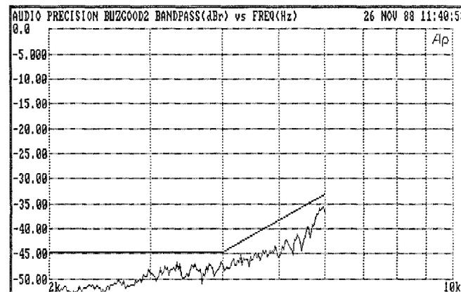
**Figure 24 Rub and Buzz Test Result, Good Tweeter #2**
