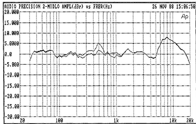
Figure 10 Two Response Tests Superimposed, One With Defective Lower-Midrange Driver
