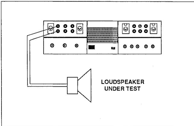
Figure 29 Connection Diagram, Impedance Tests
