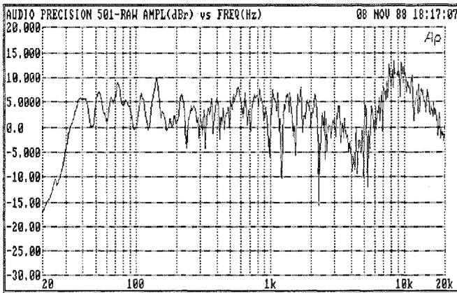
Figure 3 501-Point Measurement of Full-Range Speaker System in Reflective Space
