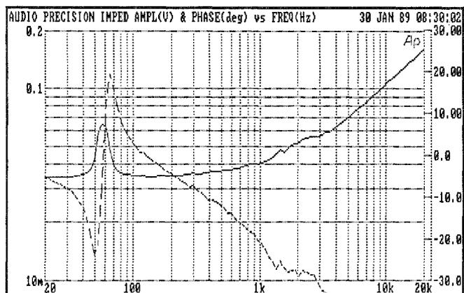
Figure 2 Driver Voice-Coil Impedance Amplitude (Solid Line) and Phase (Dashed Line) vs Frequency
