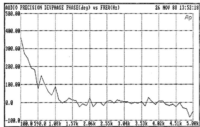
Figure 20 Deviation from Linear Phase, Obtained via COMPUTE LINEARITY Function
