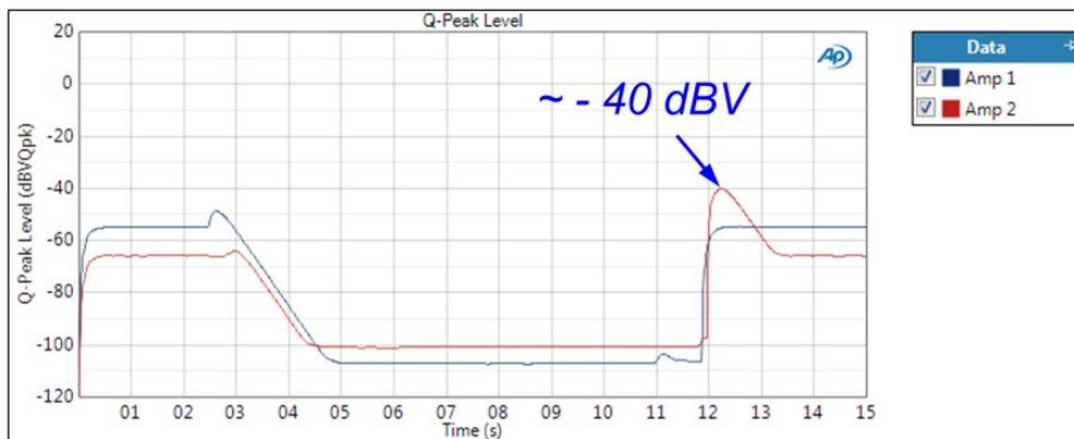
This DUT demonstrates (graph above) a maximum Q-peak level of -40 dBV. From this measurement, we can proceed with the estimation of sound pressure level.
