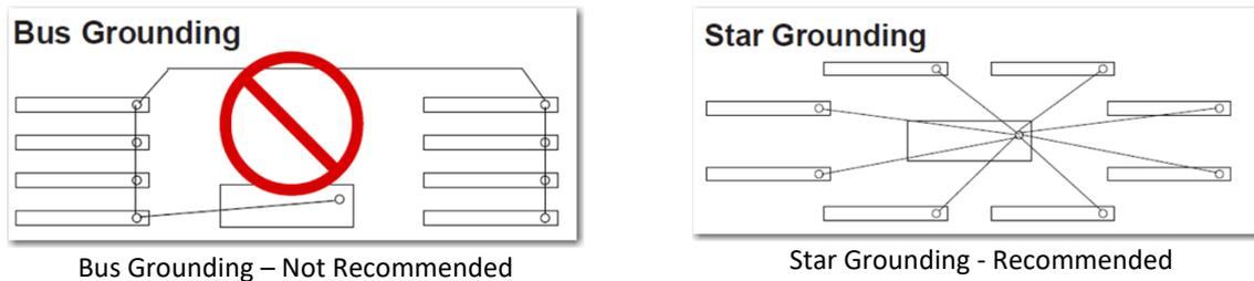
AP strongly recommends connecting the chassis ground of each device directly to the ground of the test instrument via low-impedance wires.
