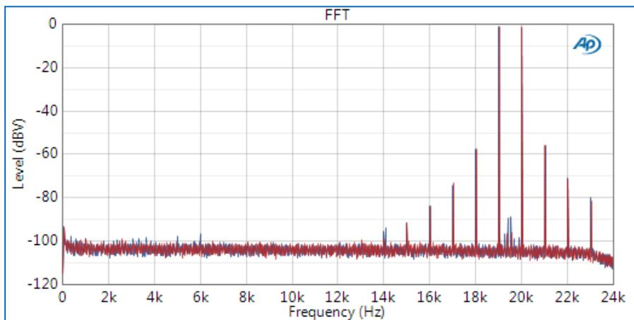
The test results for the DFD test are shown in the following figure. The 4<sup>th</sup> and 5<sup>th</sup> order products (shown as d4 and d5) are displayed in the plot for reference but are not part of the calculated ratio.
