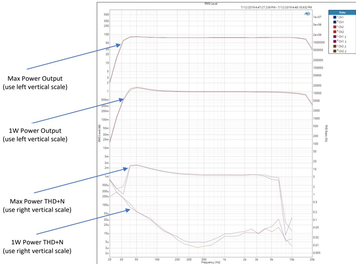
We see here that the shape of the output power curve is consistent between the power levels, but that the THD+N curves are dramatically different. Also note that both THD+N curves drop precipitously at about 6 kHz, which demonstrates that the value of this measurement is diminished when harmonics are beyond the bandwidth cutoff.
