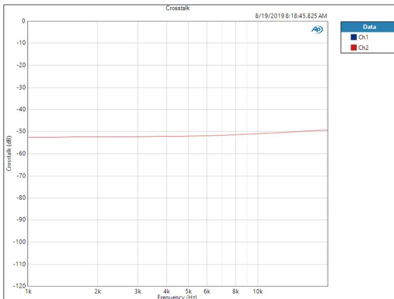
Crosstalk should be measured as a function of frequency, as it commonly varies substantially with frequency. If a single-measurement test is desired, it is commonly measured at 10 KHz. This is for two reasons. First, the
