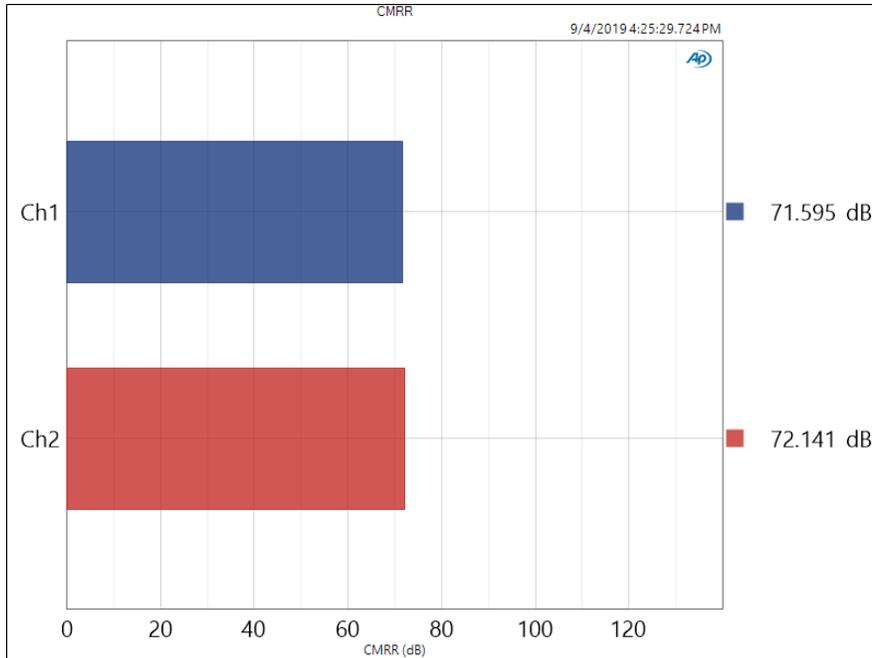
The IEC 60268-3 standard defines a slightly different implementation for the CMRR test. The differential signal is first measured and the value stored. Next, each output leg is separately measured as a common mode output with a 10-ohm source resistance in series with each leg as defined by the IEC 60268-3 specification. The higher measured common mode level of the two outputs is used as the common mode value, and finally the calculation is performed as described in the previous paragraph.
