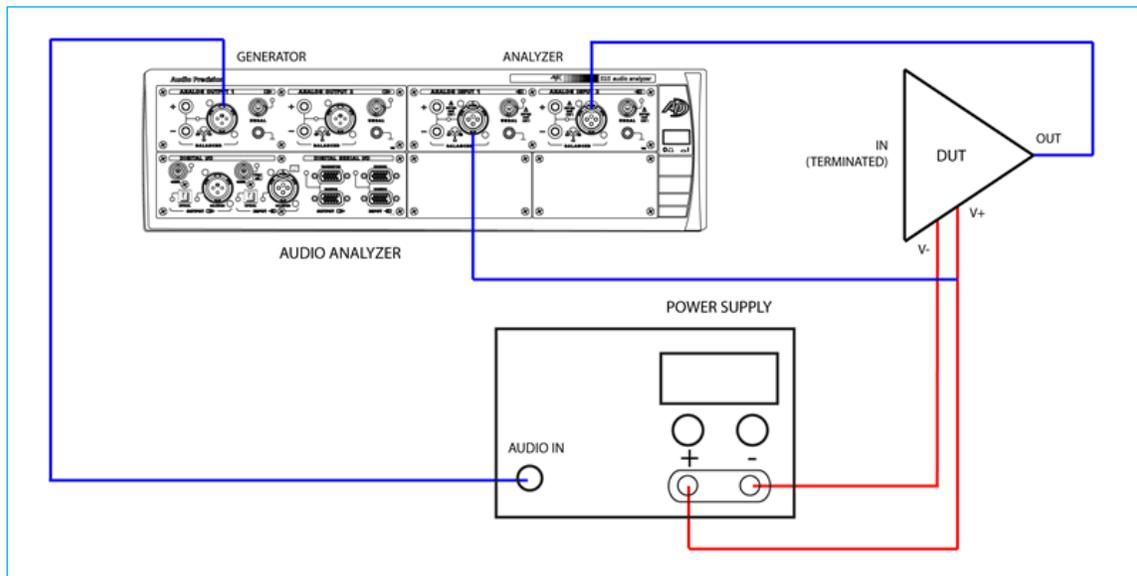
From this diagram, you can see that the output of one of the generators is connected to the modulator input (shown in the figure as AUDIO IN) of the power supply, providing the modulation for the output of the supply. Two inputs are used on the audio analyzer; one for measuring the amplitude of the signal on the DC supply output, and one to measure the related frequency on the output of the DUT. For this test, the DUT inputs are terminated.
