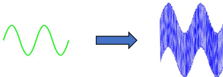
These noise signals have very high slew rates (SR), which can cause erroneous distortion and noise readings in analyzer measurements. In some cases, audio analyzer circuits can be forced into unstable states or even suffer damage.
