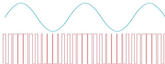
The output signal swings from maximum output to minimum output very quickly (resulting in high frequency content in the output) as can be seen in the following image.
