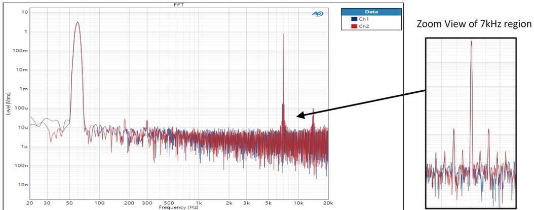
The harmonics of interest are now located near the 7 kHz tone. Any harmonics of the 60 Hz tone that are seen at 120 Hz, 180 Hz, etc., are not relevant to this test. The SMPTE IMD is then determined as the RMS level of IMD products expressed as a ratio to the RMS level of  $f_2$ . The following is a representation of the SMPTE IMD test result.
