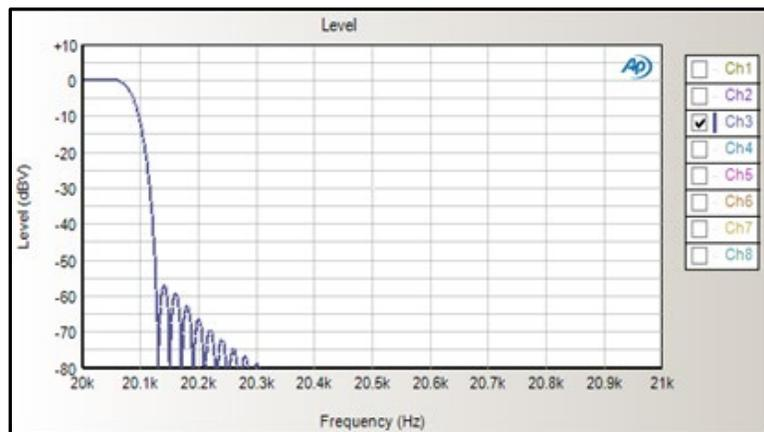
It is critical that a passive external filter be used in addition to the AES17 filter to assure good measurement quality and avoid potential damage to the analyzer input. The analyzer's internal AES17 filter does nothing to protect the analyzer input stages from effects of the high frequency content of the Class D output.
