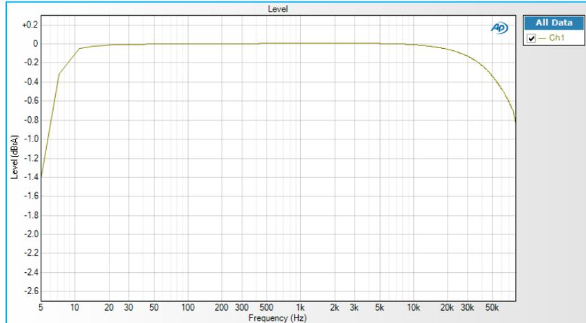
Traditionally, this test has been done with a stepped frequency source. However, especially in environments such as production test, much of this work is now done using a logarithmically-swept sine (chirp) signal to substantially reduce test time. A 23-second stepped-frequency test, for example, can be replaced with a 4-second chirp test with comparable results.
