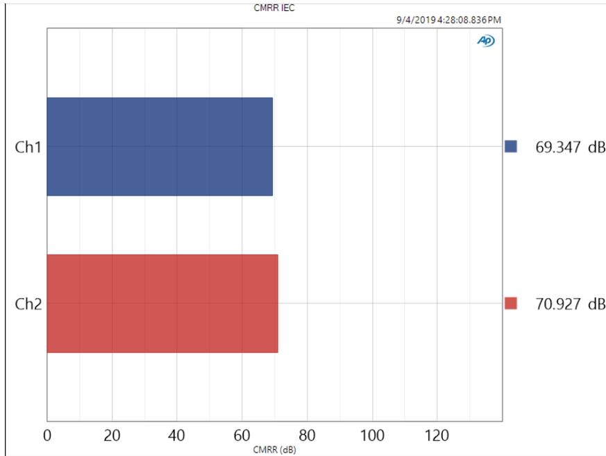
For a well-designed amplifier, these CMRR test results are typically in the 60 dB or greater range. You can see that the IEC CMRR method is slightly more pessimistic than the basic CMRR test. The Audio Precision APx500 audio analyzers (B Series or Legacy) are designed to perform either of these CMRR tests, which can be selected from the list of available measurements.
