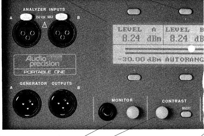
stacks who counting st bual output generator drives channel A, B, or A&B at touch of a button without moving cables.
