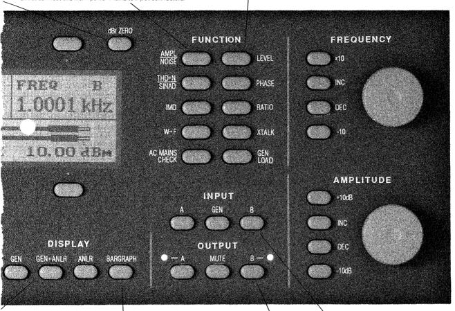
PRSQUEMCY: Increase/ decrease generator frequency (or analyzer selective filter frequency in selective analysis mode) in 10x steps, ½ octave steps, or continuously variable via knob with 0.02% resolutior.
