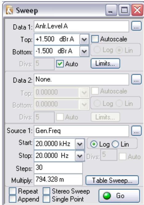
For a more useful display of the same data, you can set the Analyzer dBr input reference to your 1 W level. This will display 0 dB at the center frequency of 1 kHz, if you set the Sweep units to dBrA. You can also adjust the graph axis scales for a more useful display. Since our DUT is quite flat, we can narrow the view to just a few decibels above and below the reference.
