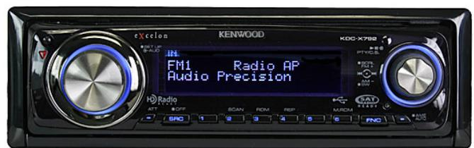
Figure 12. Radio receiver displaying RDS text.
