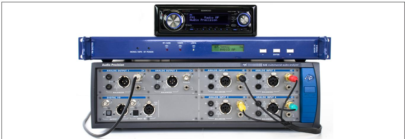
Figure 1. FM radio test setup, with APx526, transmitter, and car stereo.
