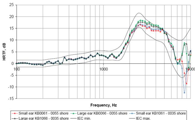
Figure 3. HRTFs for the KEMAR 45BA manikin with different styles of pinnae.
