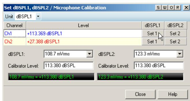
Figure 8. Setting the dB SPL reference levels.
