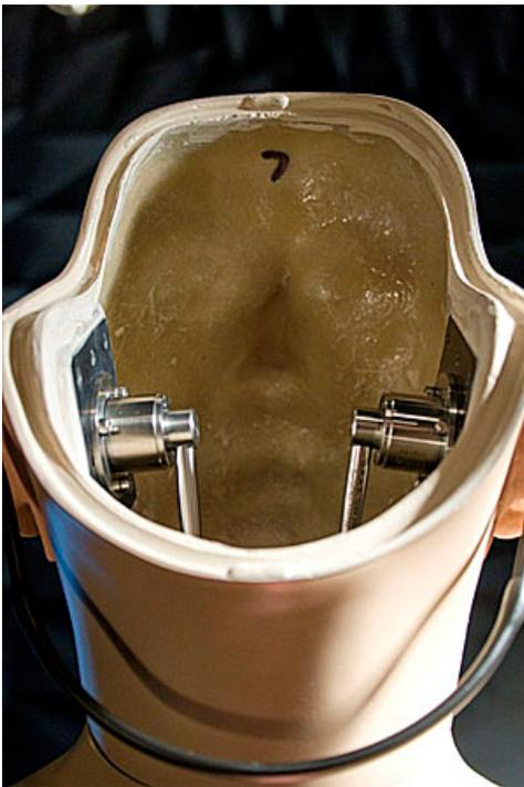
Figure 2. Ear simulators and microphones inside the head of the HATS.
