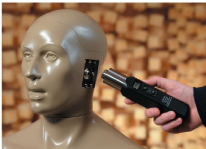
Figure 7. Calibrating the microphones.
