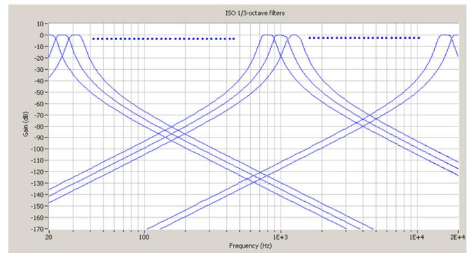
Figure 6. Derivation of the 1/3-octave spectrum from the FFT.
