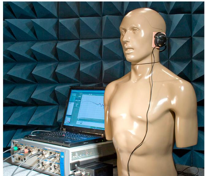
Figure 1. APx526 audio analyzer with G.R.A.S. KEMAR manikin type 45BA.
