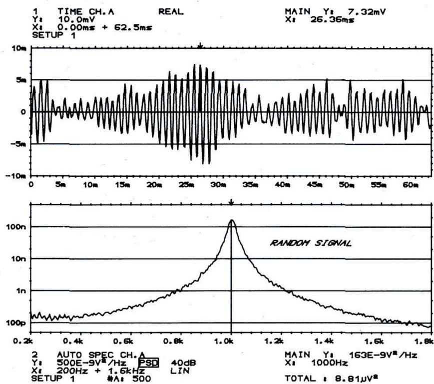
Fig. 1. Time record and frequency spectrum for a stationary, random process. The frequency spectrum is scaled as the power spectral density.
