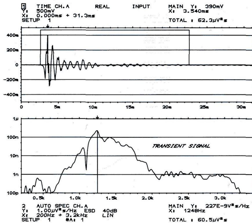
Fig. 2. Time record and frequency spectrum for a transient signal. A transient time-weighting function is used in the analysis of the time record, and the frequency spectrum is scaled as the energy spectral density.
