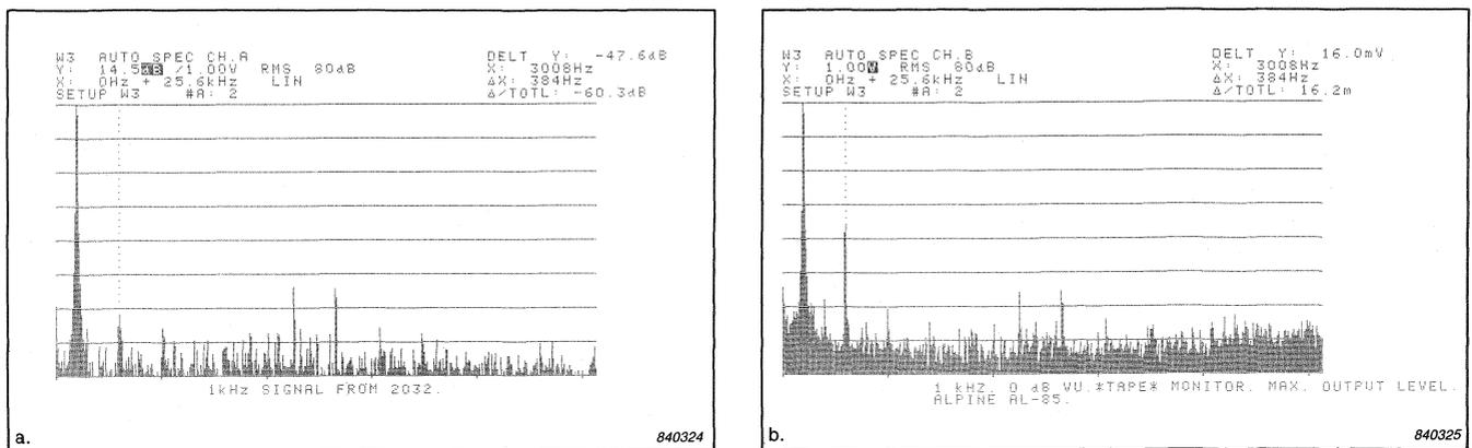
Fig. 23. (a) The built-in sine generator of Types 2032 and 2034 is of good quality. Its distortion products lie generally below -60dB, which is sufficient for measurements on most tape recorders\*
