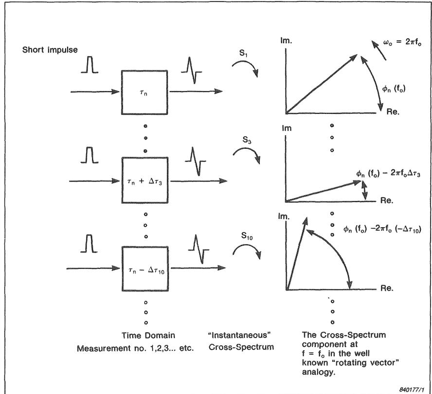
Fig. 3. The influence of test object delay-variation on the "instantaneous" cross spectra
