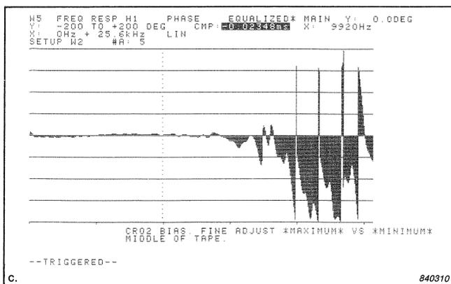
Fig.13. Movement of recording zone as function of bias level. Neglecting the influence of tape speed drift, the movement amounts to  $23,5 \mu s \times 4,76 \text{ cm/s} = 1,1 \mu m$ . The nominal head gap-width is  $3 \mu m$
