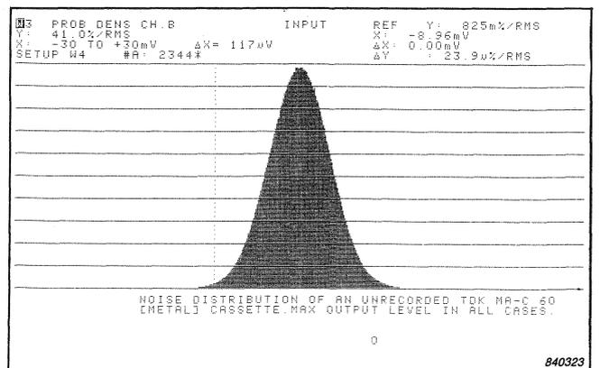
Fig. 22. The Analyzer in its statistical mode
