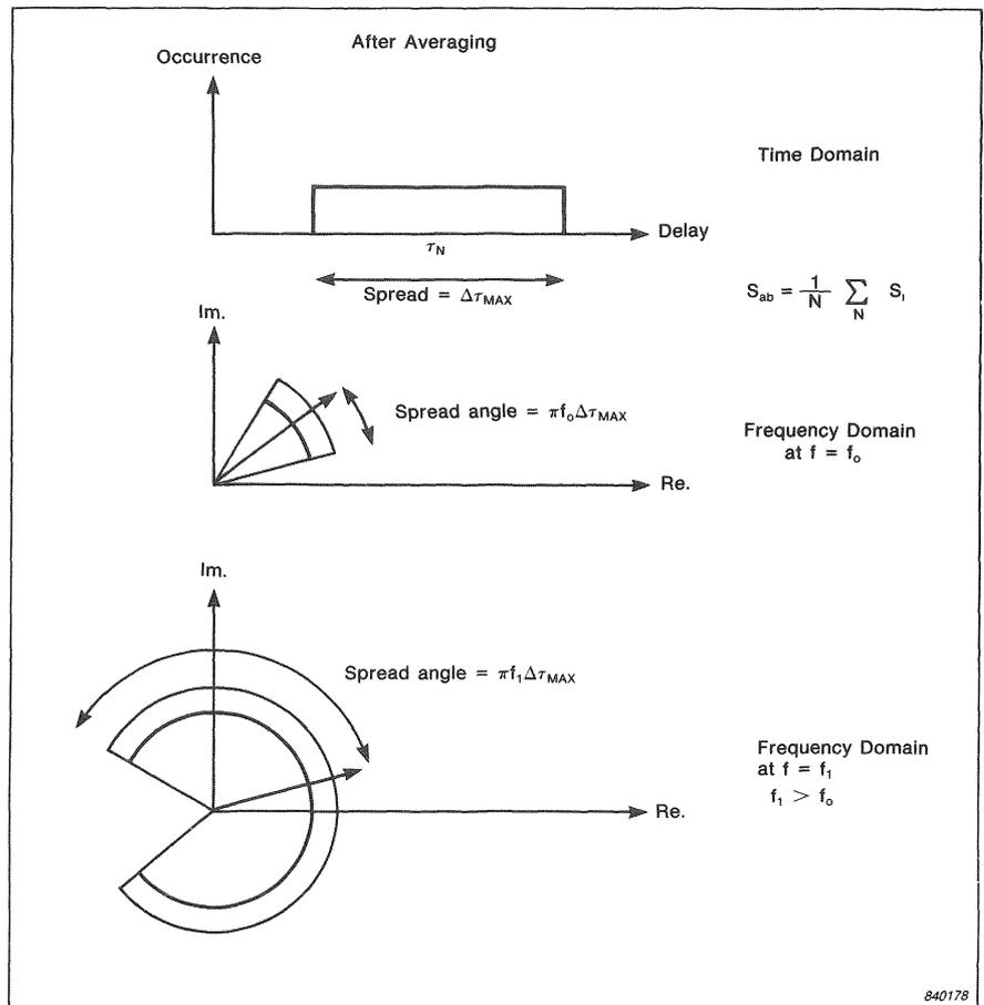
Fig. 4. The spread of the encountered delays causes spread in the direction of the encountered cross-spectrum components
