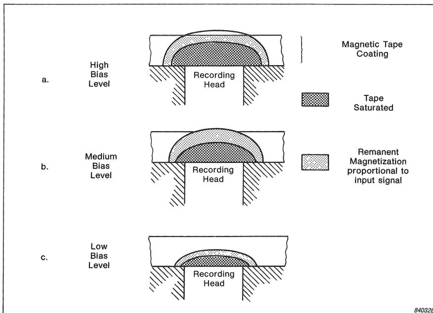
Fig.12. The recording zones present in front of a recording head at:
