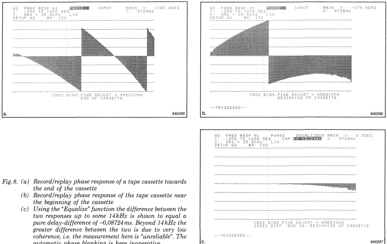
Fig.8. (a) Record/replay phase response of a tape cassette towards the end of the cassette
