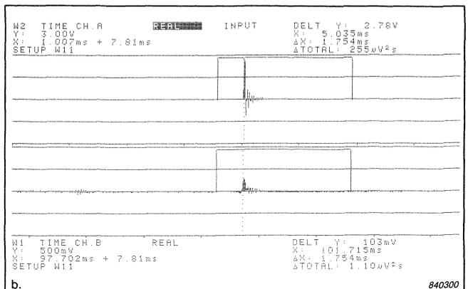
Fig.7. (a) The recorded impulse (bottom) when the input impulse (top) is band-limited to 20kHz
