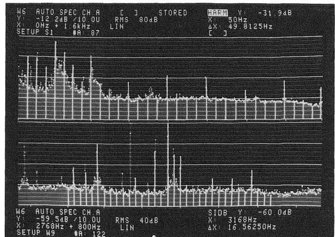
\* An external, higher quality sine generator may be employed to provide full utilization of the 80dB dynamic range of the Analyzers. At frequencies above 12kHz the harmonic distortion can no longer be measured. Twin tone difference frequency distortion can then be employed, using both the external sine generator and the built-in generator of Type 2032/34
