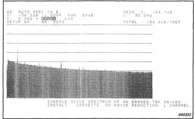
The basic tape noise is due to random orientation of the small magnetic particles in the tape causing a varying flux through the replay head. Generally the higher the density of particles, the less the flux variation and hence the less is the noise.
