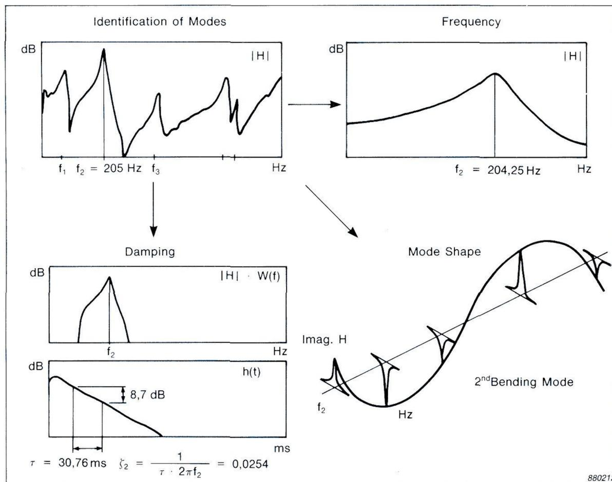
The frequency response function of a structure can be separated into a set of individual modes. By using a Dual-Channel Signal Analyzer Type 2032 or 2034, each mode can be identified in terms of frequency, damping and mode shape.
