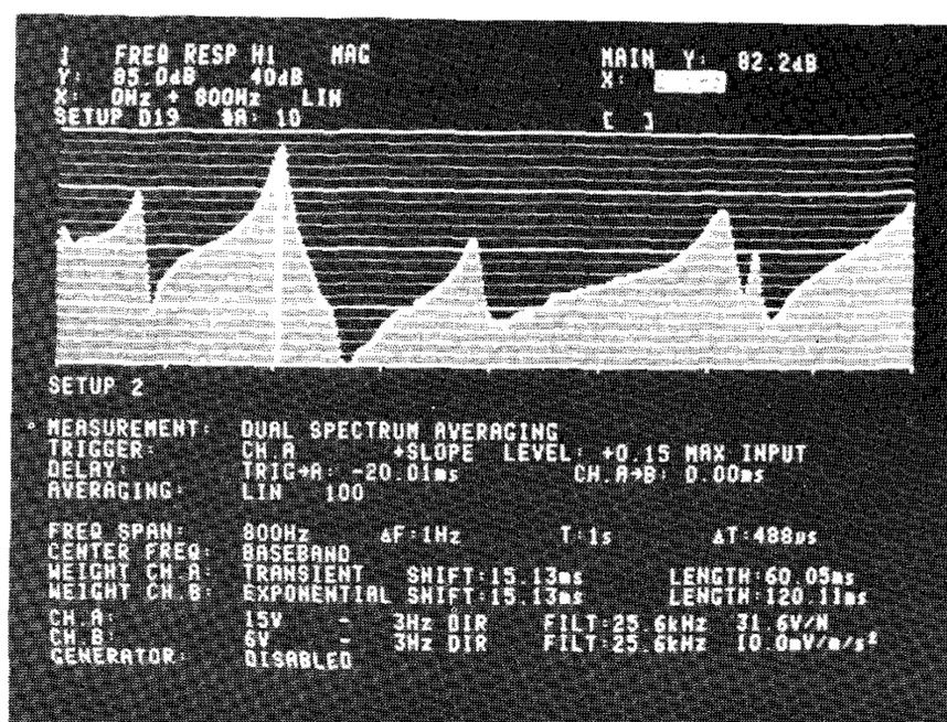
Fig. 3. Magnitude of the frequency response function for the test structure.
