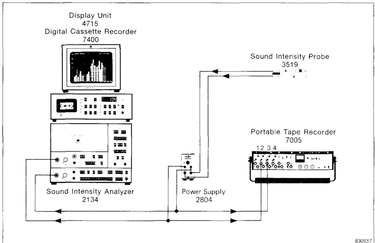
Fig.14. Measurement set-up for simultaneous analysis and tape recording of sound intensity
