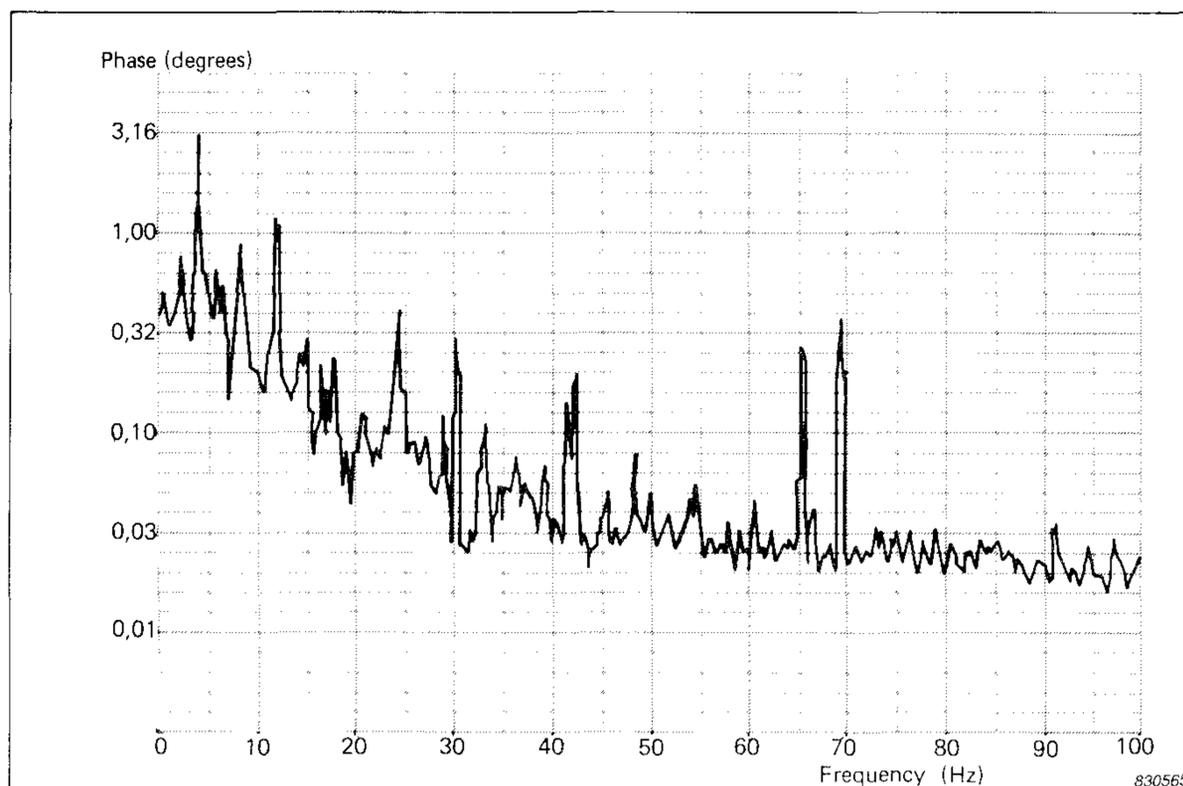
Fig.7. Spectrum of relative phase fluctuations between channel 1 and 4 measured by recording a 10kHz signal in both channels at a tape speed 381 mm/sec and passing the outputs through a phasemeter and frequency analysing the phase fluctuations. The sharp peaks can be related to the dimensions of the wheels of the tape transport system
