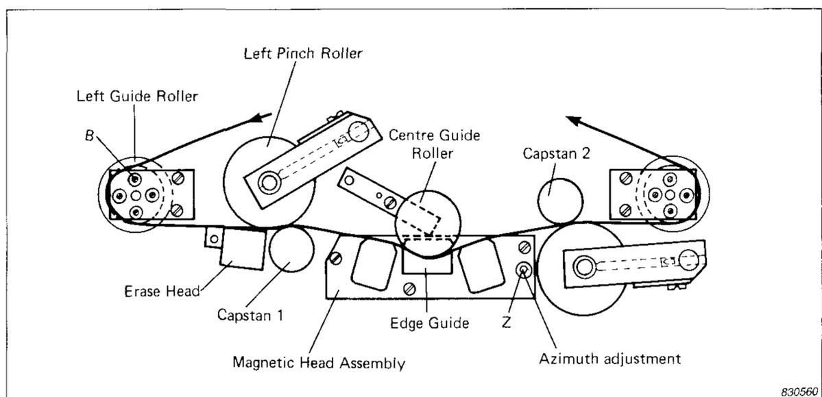
Fig.13. Tape transport and the magnetic head assembly under the front cover. Azimuth adjustment is performed by gently turning screw Z
