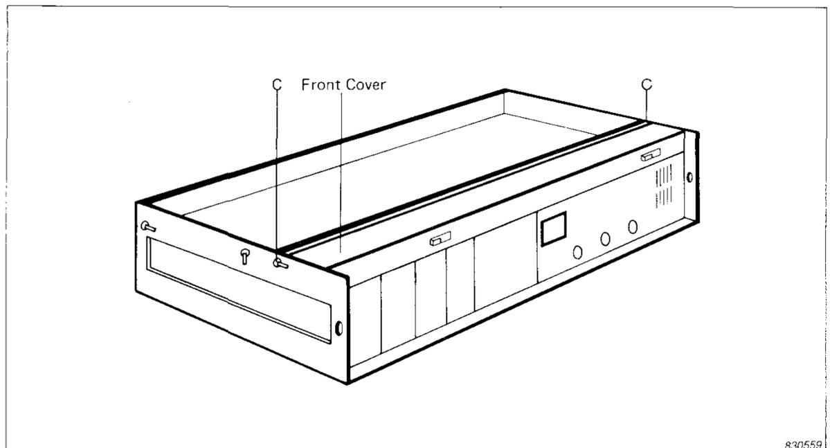
Fig.12. Chassis of the Tape Recorder Type 7005 showing the screws which secure the front cover
