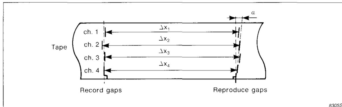
Fig.5. Record gaps and reproduce gaps in a 4-channel tape recorder
