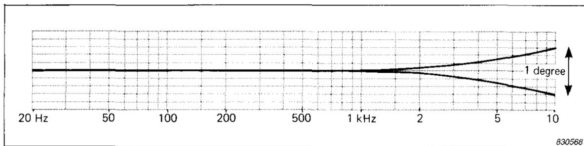
Fig.4. Typical relative phase-mismatch between two channels using FM recording with optimal azimuth adjustment
