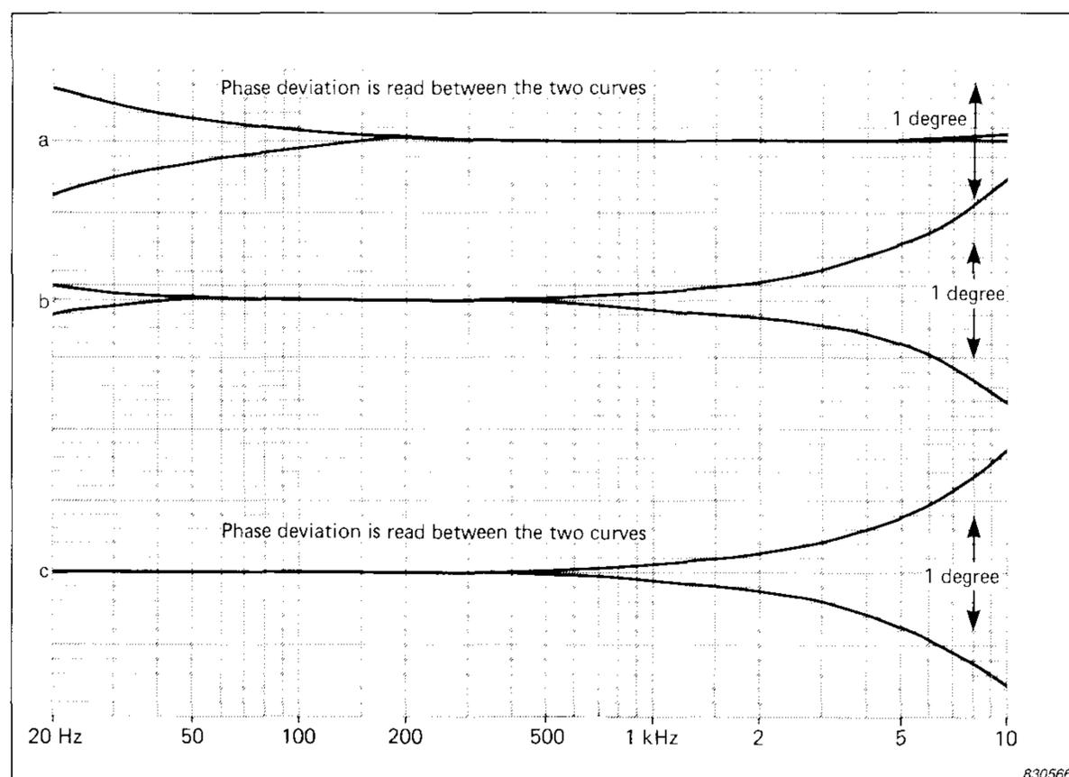
Fig.2. Typical relative phase-mismatch in two record — reproduce amplifiers
