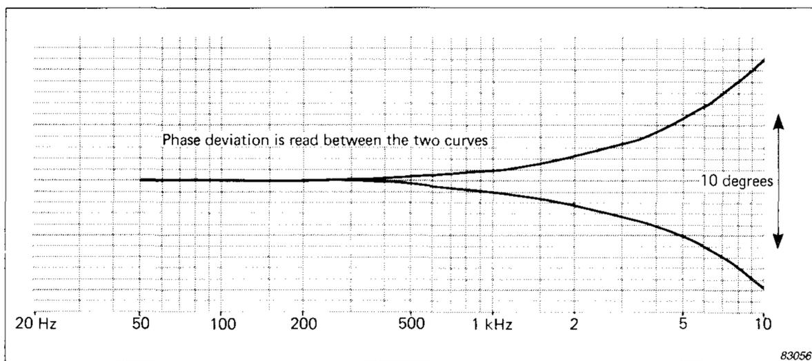
Fig.6. Relative phase-mismatch between two channels using FM recording with non optimal azimuth adjustment
