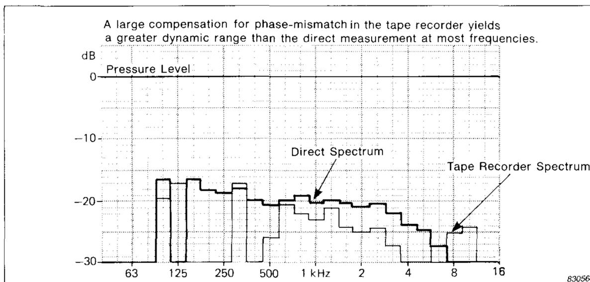
Fig.11. Pressure, direct intensity and tape recorded intensity spectrum for 4 different azimuth adjustments. Dynamic range of the system is in each case the difference between pressure and intensity levels
