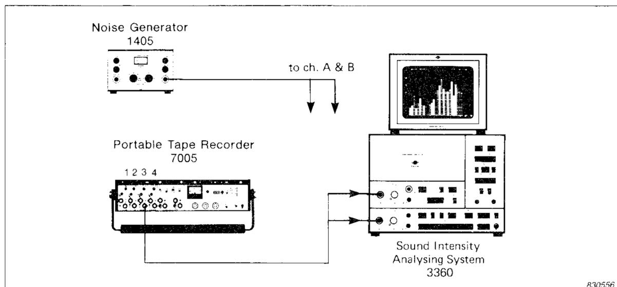
Fig.9. The dynamic range of the analyser alone (without the probe) can be checked by putting the same noise signal into both channels simultaneously. This simulates a diffuse field. Alternatively a reference signal may be taken from one channel of the record/reproduce units of the Tape Recorder
