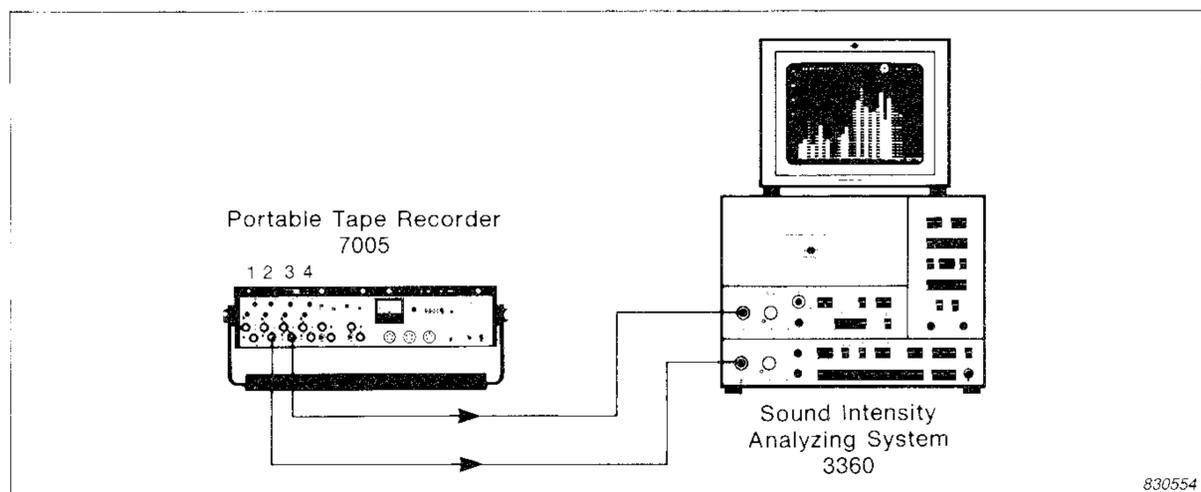
Fig.10. Set-up for analysis of the tape recorded Intensity measurement
