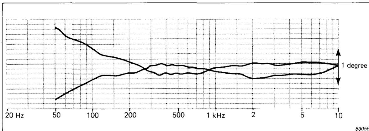
Fig.3. Typical relative phase-mismatch between two channels using direct recording with optimal azimuth adjustment
