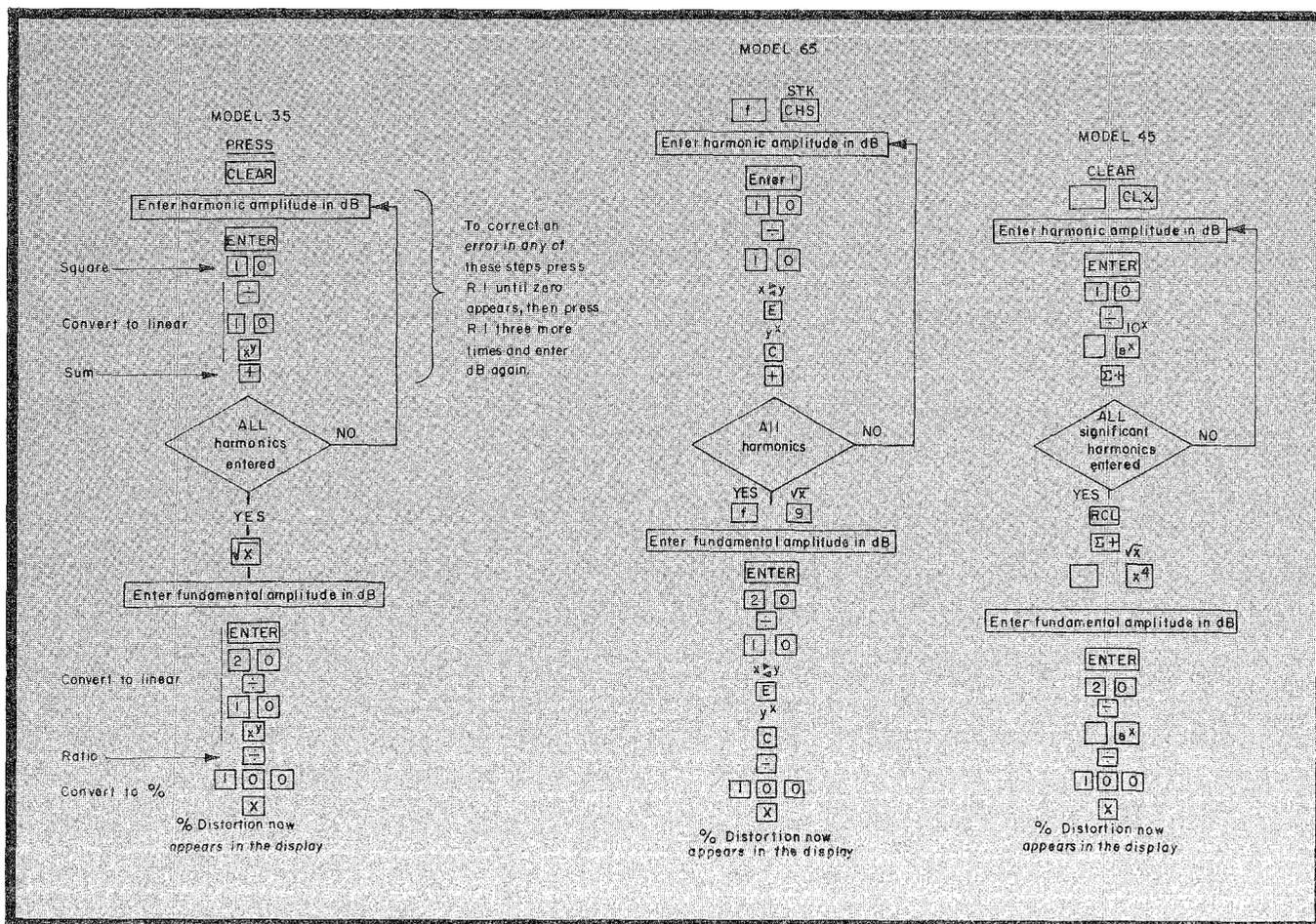
Figure 2. Three harmonic distortion algorithms using HP calculators.
