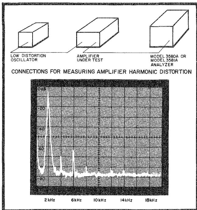
Figure 3. Measurement results show total harmonic distortion to be greater than 63 dB below the fundamental.
