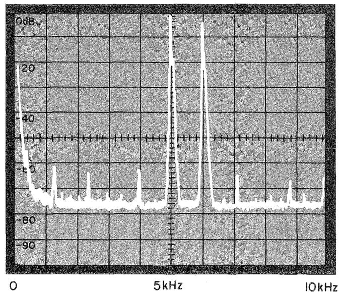
Figure 7. Distortion measurement using the CCIF method.
