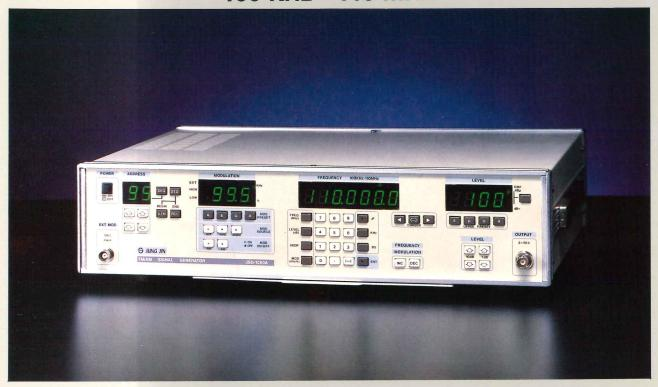
The Model JSG-1050A is a standard signal generator that covers the frequency range, 100kHz to 110MHz, for AM and FM signals suitable for testing multiband radios and in CB, cordless telephone production line. Modulation can be selected to 0 to 60% at AM, and 0 to 99.5kHz at FM.
