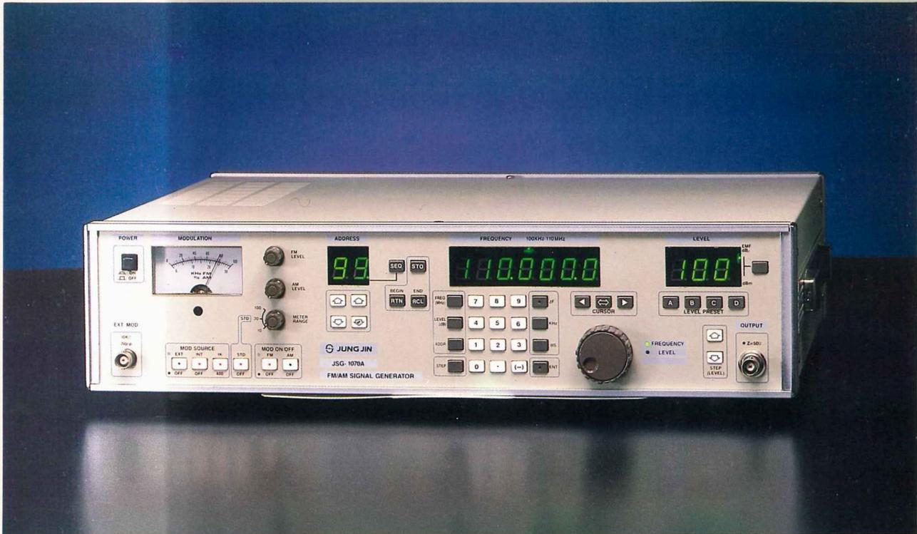
The Model JSG-1070A is a standard signal generator that covers the frequency range, 100kHz to 110MHz, for AM and FM signals suitable for testing multiband radios and in CB, cordless telephone production line. Modulation can be controlled 0 to 60% at AM, and 0 to 100kHz at FM.
