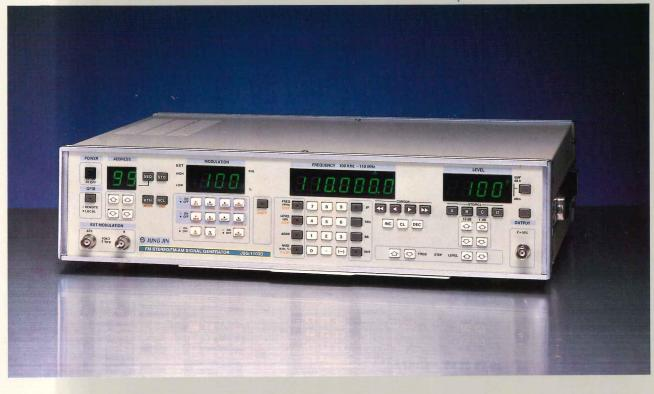
The JSG-1100B is a versatile instrument, specially developed and designed to generate FM and AM signals as well as FM stereo signals used in the radio production line. The carrier frequency range covers 100 kHz to 110MHz and the FM stereo band, 75 to 110 MHz. PLL system is employed for high accuracy and stability in generation of the carrier frequencies. All operating functions are microprocessor-controlled and set values are displayed digitally.
