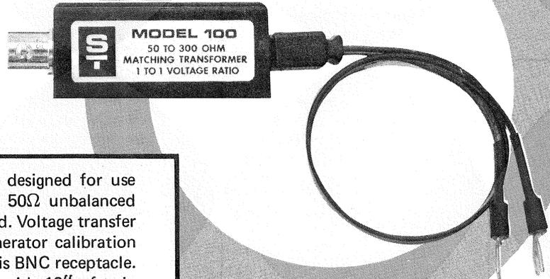
The Model 100 Matching Transformer, designed for use from 54 MHz to 216 MHz, converts a 50Ω unbalanced signal generator output to 300Ω balanced. Voltage transfer ratio is 1:1 ± 10%, retaining signal generator calibration into a 300Ω load. 50Ω input connector is BNC receptacle. Detachable 300Ω output plug is wired with 12" of twin lead terminated in spade lugs.
