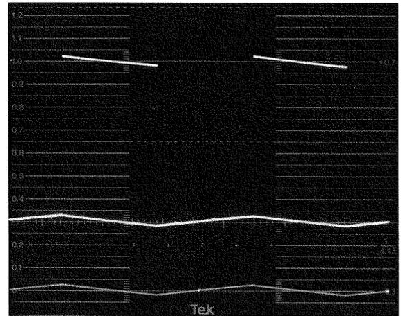
Figure 34. A 2-field waveform monitor display showing field time distortion.
