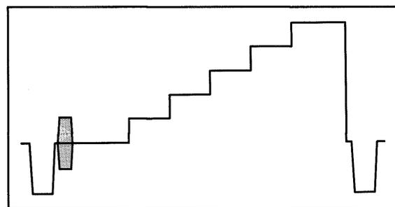
Figure 109. A signal which extends to 700 mV, such as this Staircase signal, is used in conjunction with the zero carrier pulse to verify modulation levels.
