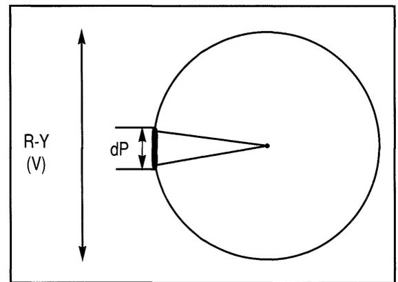
Figure 66. Differential phase distortion affects the R-Y (V) signal.
