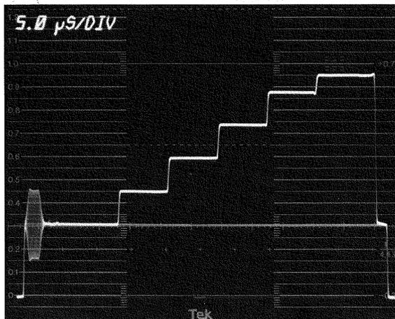
Figure 81. An example of luminance non-linearity distortion.
