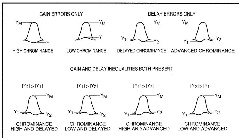
Figure 23. Effects of gain and delay inequalities on the modulated sine-squared pulse.
