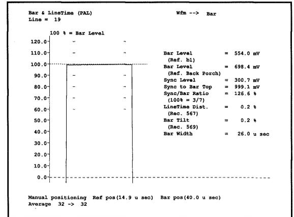
Figure 32. The VM700A Bar LineTime display.
