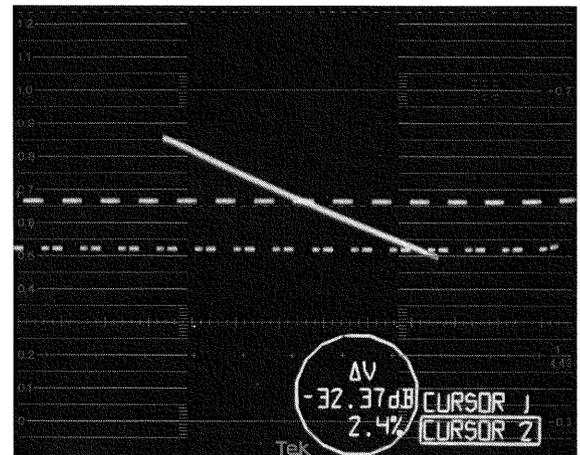
Figure 35. The 1781R voltage cursors can be used to measure field time distortion.
