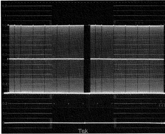
Figure 42. 6 MHz field-rate sweep signal with markers (2-field display).
