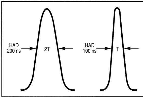
Figure 111. 2T pulse and 1T pulses for PAL systems.
