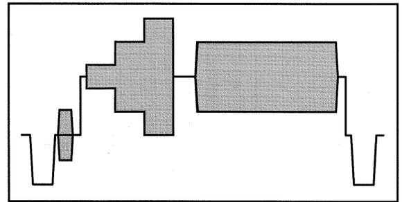
Figure 90. This combination ITS contains the Modulated Pedestal signal element (CCIR Line 331).
