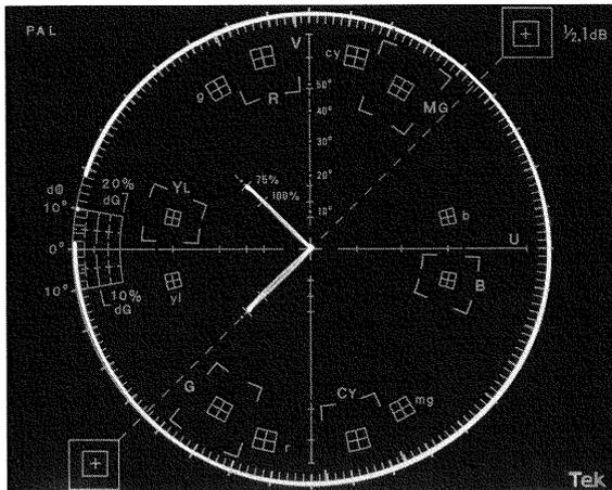
Figure 19. The 1781R's polar SCH phase display, showing a 10 degree error.
