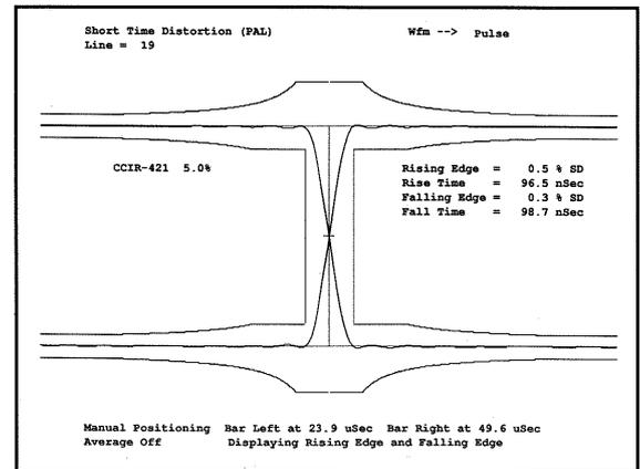
Figure 29. The VM700A Short Time Distortion display.
