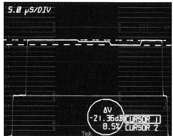
Figure 91. A chrominance-to-luminance intermodulation distortion of 8.5% referenced to the pedestal level.
