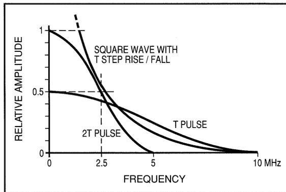
Figure 113. Frequency spectra of T pulse, 2T pulse, and T step.
