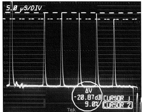
Figure 82. This photograph shows a 5 step Staircase after it has been passed through a differentiated step filter. The 1781R voltage cursors indicate 9% luminance non-linearity.
