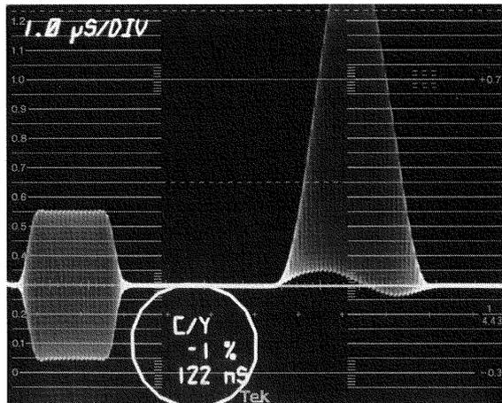
Figure 25. Results obtained with the CHROMA/LUMA selection in the 1781R's MEASURE mode.
