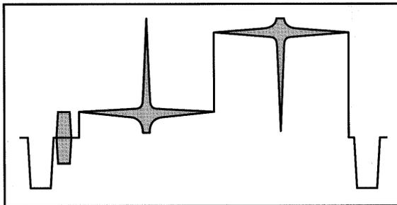
Figure 43. Time domain display of Sin X/X.
