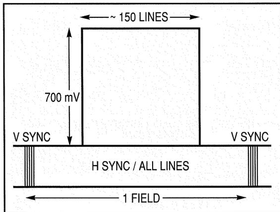
Figure 33. The Field Square Wave test signal.
