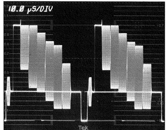
Figure 2. A waveform monitor display of Colour Bars; 2-line display.
