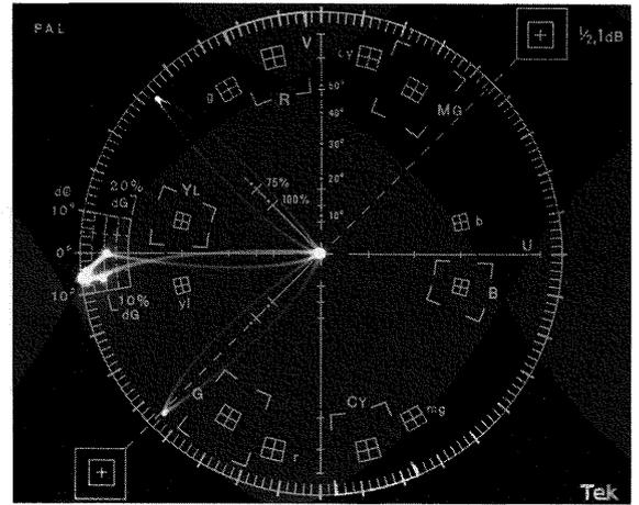
Figure 72. A vectorscope display of a signal with 10% peak-to-peak differential gain. (Differential phase distortion is also present.)
