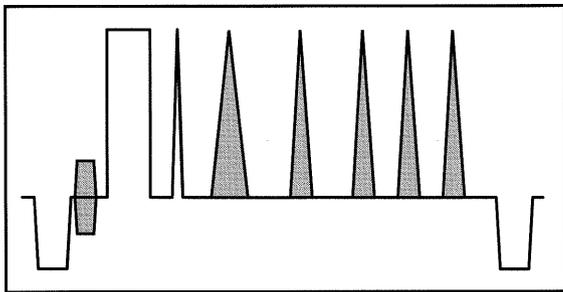
Figure 51. The Multipulse test signal.
