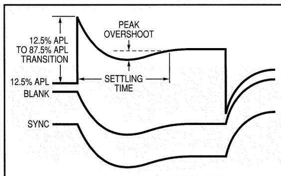
Figure 38. Long time distortion measurement parameters.
