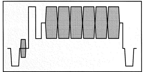
Figure 40. A Multiburst test signal.
