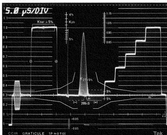
Figure 61. This signal is properly positioned for a  $K_{\text{bar}}$  measurement with the 1781R graticule.
