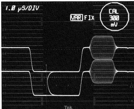
Figure 10. The WFM + CAL mode can also be used to measure sync amplitude.
