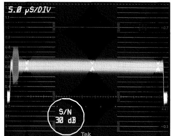
Figure 99. Properly adjusted separation; this signal has a signal-to-noise ratio of 30 dB.
