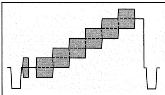
Figure 71. A Modulated 5-step Staircase test signal.
