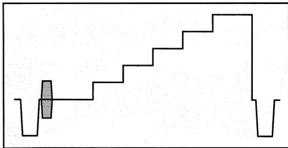
Figure 80. Unmodulated Staircase signal.
