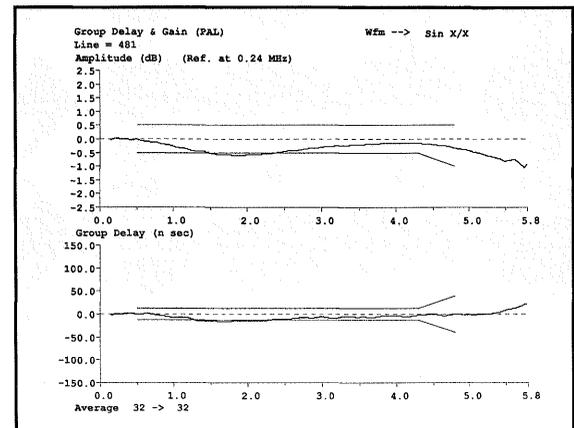
Figure 50. VM700A Group Delay Sin X/X measurement.
