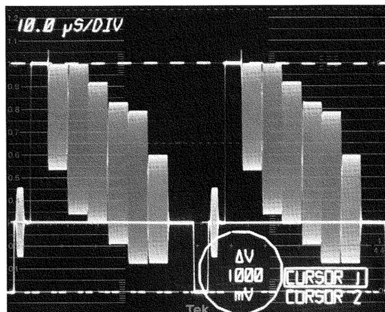
Figure 11. 1781R voltage cursors positioned to measure peak-to-peak amplitude.
