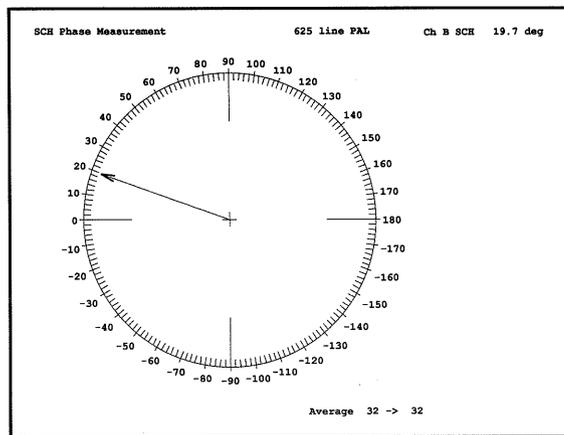
Figure 20. The VM700A SCH Phase display.
