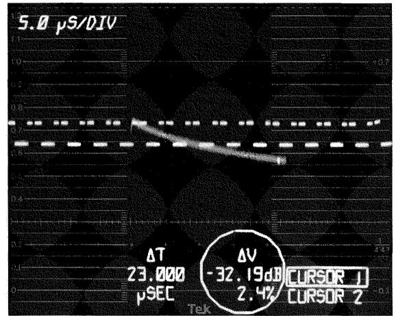
Figure 31. The 1781R voltage and time cursors can facilitate line time distortion measurements.
