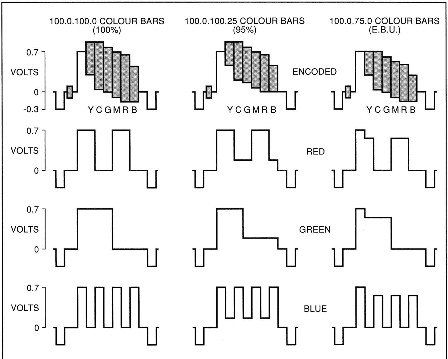
Figure 110. Waveforms and RGB voltages for three types of PAL colour bars.
