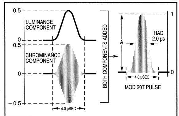
Figure 22. The chrominance and luminance components of a modulated sine-squared pulse.
