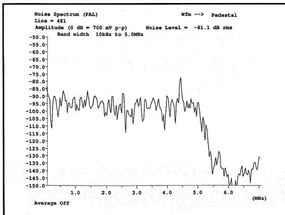
Figure 100. The VM700A Noise Spectrum display.
