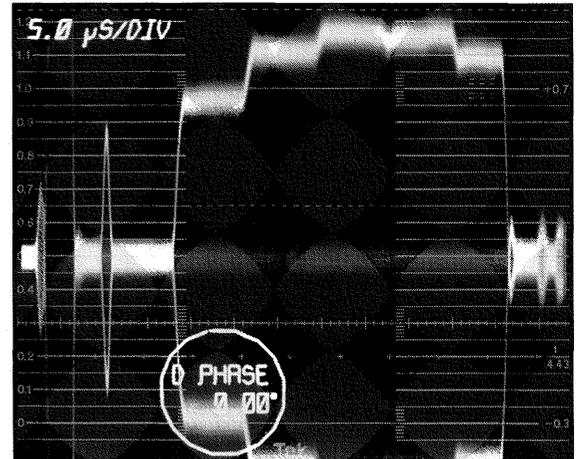
Figure 68. The 1781R double trace DIFF PHASE display; phase readout zeroed.
