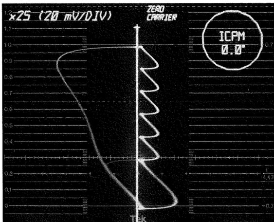
Figure 103. 1781R display; no ICPM distortion.
