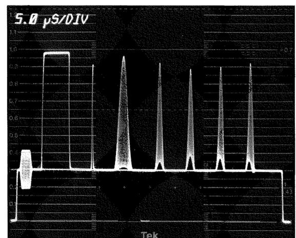
Figure 46. Multipulse exhibiting frequency response distortion.
