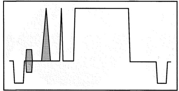
Figure 57. This signal contains the pulse and bar signal elements required for K Factor measurements.
