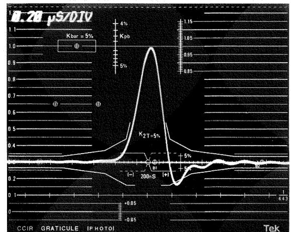
Figure 58. A 2T pulse properly positioned for a  $K_{2T}$  measurement. This signal has a  $K_{2T}$  distortion of slightly more than 5%.
