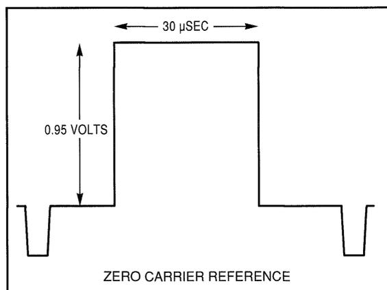
Figure 108. The zero carrier reference pulse as it appears in a baseband signal.
