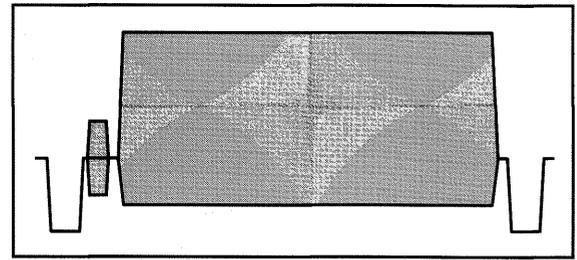
Figure 97. The Red Field test signal.
