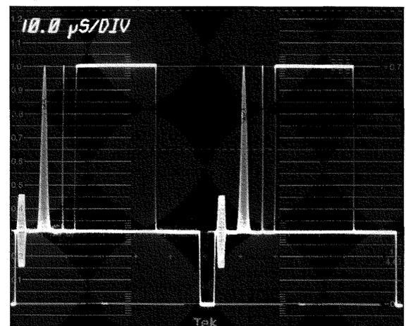
Figure 8. A 1-volt signal properly positioned with respect to the 1781R graticule.
