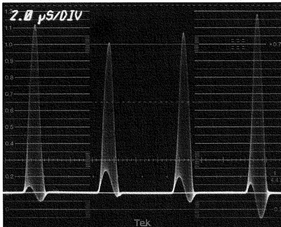
Figure 52. Multipulse exhibiting group delay distortion. Group delay differences between the high-frequency and low-frequency components of the pulse appear as sinusoidal distortion of the baseline.
