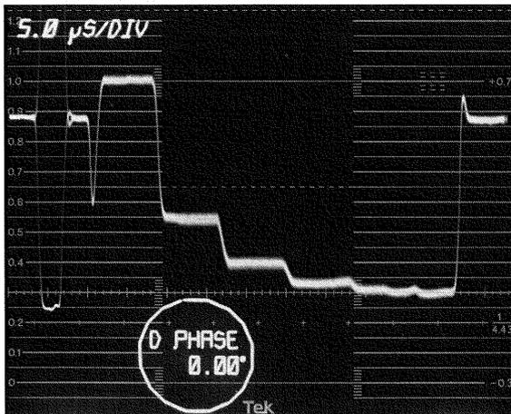
Figure 67. A single trace display indicating about 7 degrees of differential phase distortion.
