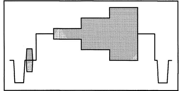
Figure 87. The Modulated Pedestal test signal.
