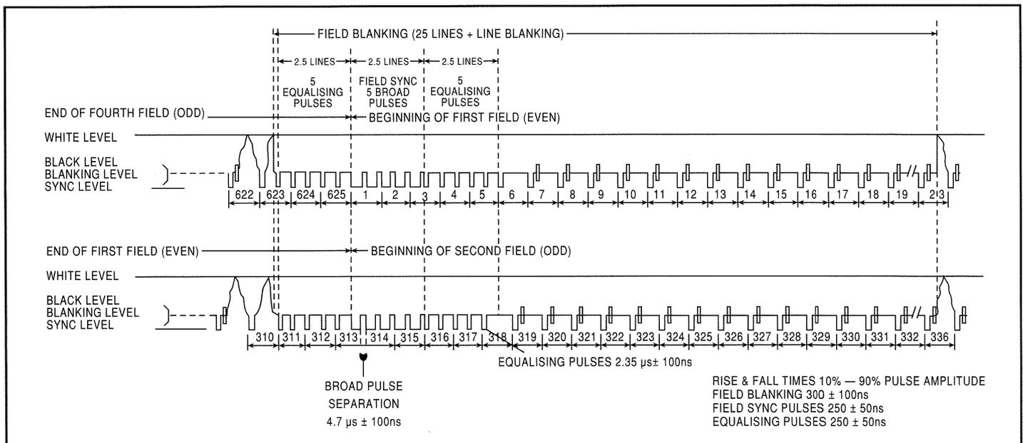
Figure 18. CCIR vertical interval specifications.
