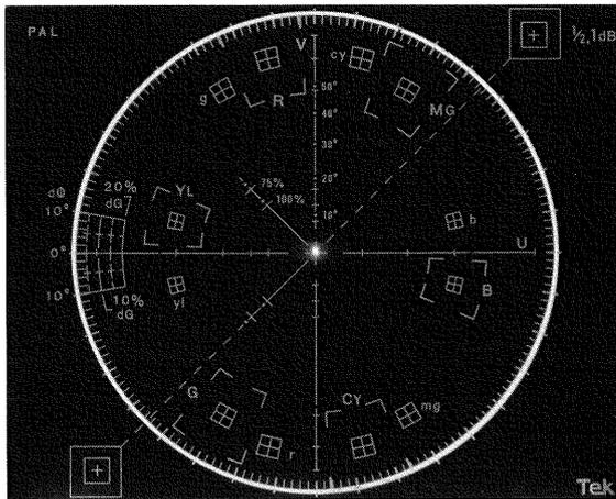
Figure 5. The 1781R vectorscope calibration oscillator.
