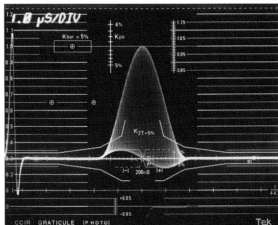
Figure 26. The 1781R graticule indicates that this signal has approximately 200 nanoseconds of chrominance-to-luminance delay.
