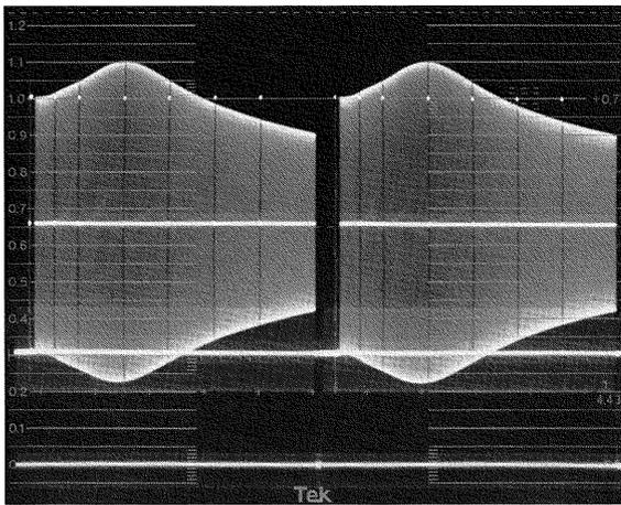
Figure 47. A sweep signal showing frequency response distortion.
