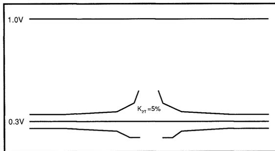
Figure 56. The 1781R's external graticule includes a 5%  $K_{2T}$  limit.
