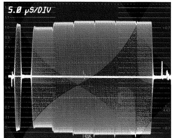
Figure 73. A chrominance filter display indicating about 6% differential gain.
