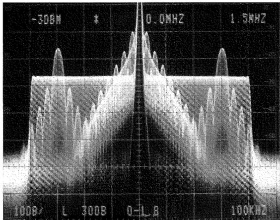
Figure 48. A spectrum analyser display of the Sin X/X signal.
