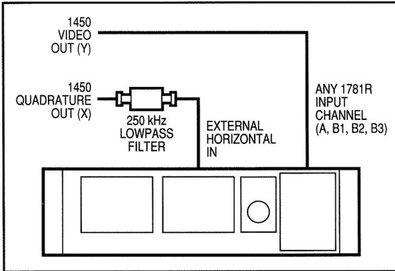
Figure 102. How to hook up the 1781R for ICPM measurements.
