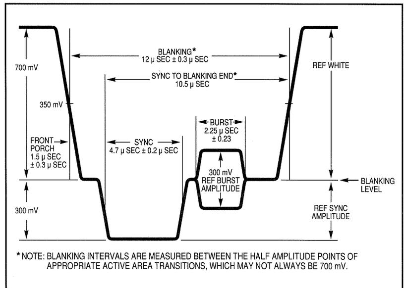
Figure 12. CCIR horizontal pulse width requirements.
