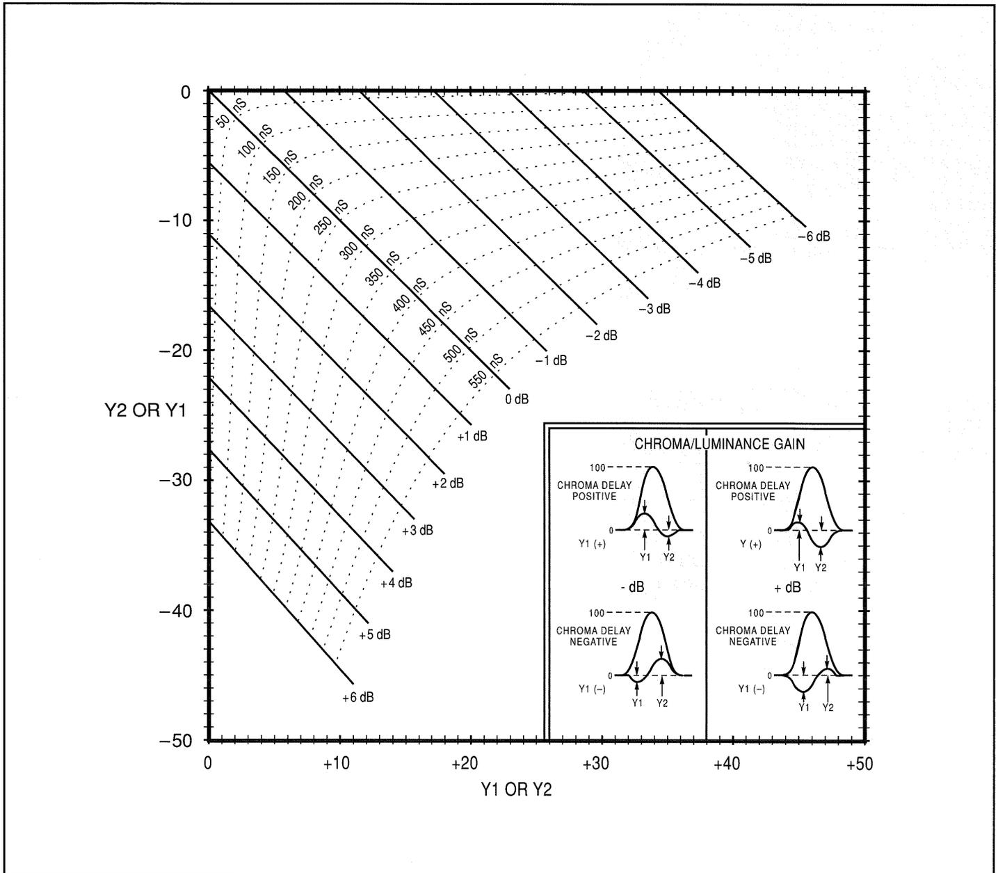
Figure 24. Chrominance-to-luminance gain and delay nomograph for a 20T pulse.
