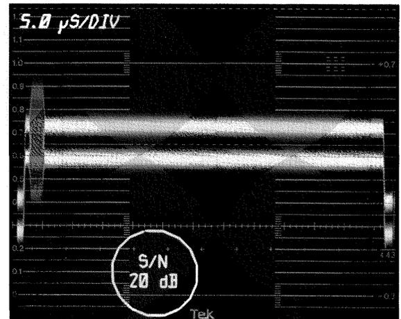
Figure 98. The 1781R tangential noise measurement mode, showing excessive trace separation.
