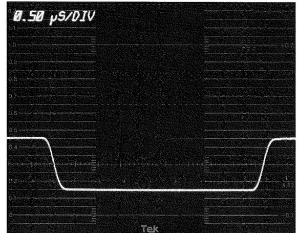
Figure 13. Horizontal sync width measurement at the 50% amplitude points.
