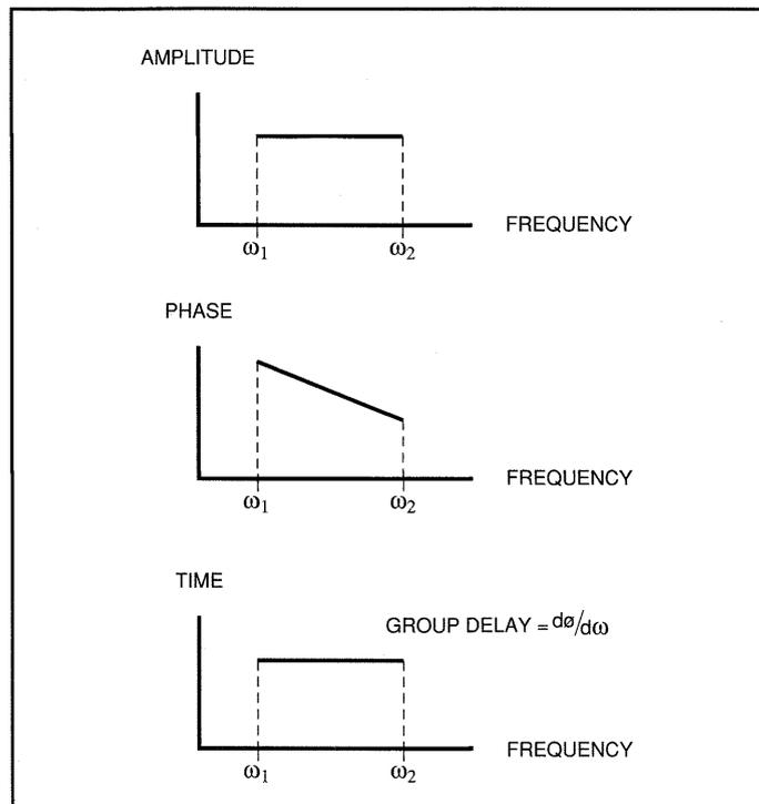
Figure 54. Response of a distortionless system.
