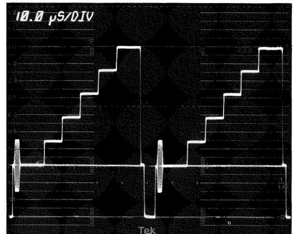
Figure 95. The sync pulse measures 300 mV at 50% APL.
