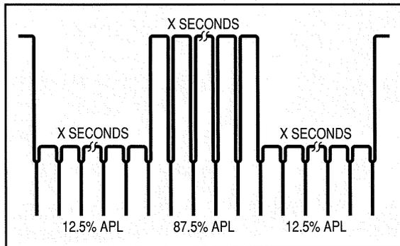
Figure 37. A Flat Field Bounce signal.
