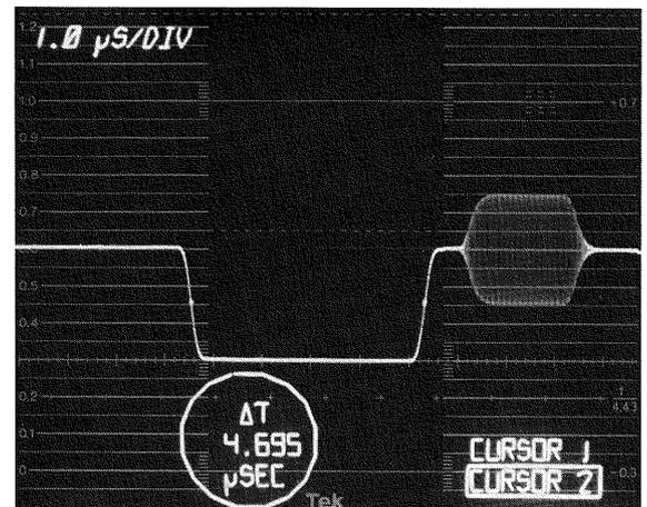
Figure 14. The 1781R time cursors positioned to measure horizontal sync width at the 50% amplitude points.
