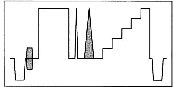
Figure 21. A combination signal which includes a 20T modulated pulse (CCIR Line 17).
