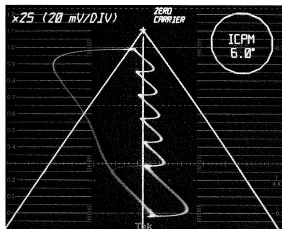
Figure 104. 1781R electronic graticule indicating an ICPM distortion of 6 degrees.
