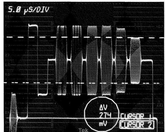
Figure 45. The peak-to-peak amplitude of the smallest packet is then measured.
