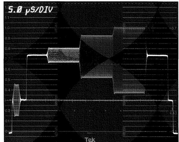
Figure 88. This signal exhibits chrominance non-linear gain distortion. Note that the amplitude of the largest packet is reduced.
