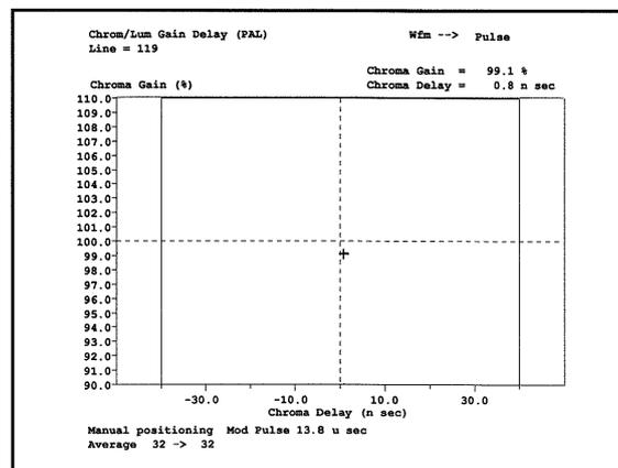
Figure 27. The ChromLum GainDelay display in the VM700A MEASURE mode.
