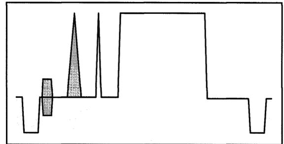
Figure 7. Pulse & Bar test signal.
