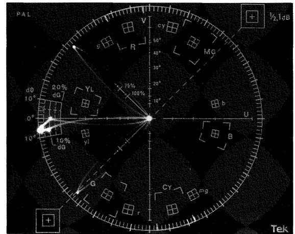
Figure 65. A vectorscope display showing a peak-to-peak differential phase distortion of about 7 degrees. (Differential gain distortion is also present.)
