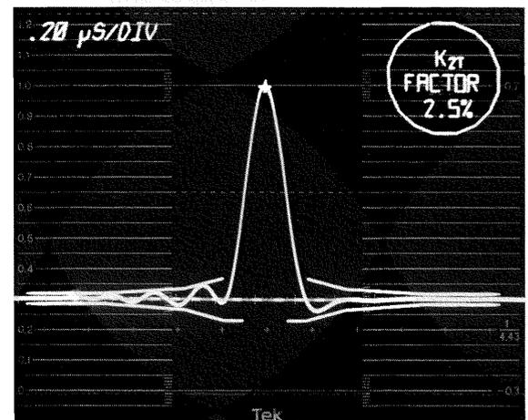
Figure 59. The 1781R electronic K Factor graticule measures a 2.5%  $K_{2T}$  distortion for this signal.
