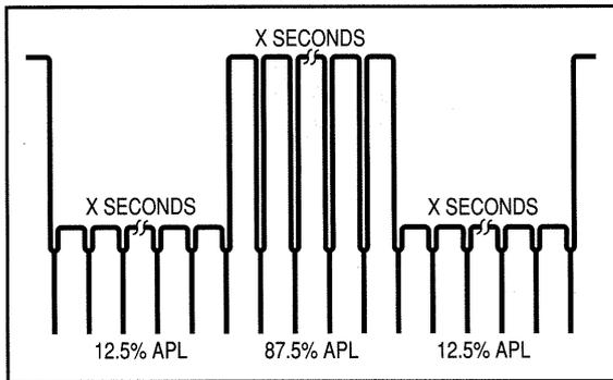
Figure 93. Flat Field Bounce test signal.
