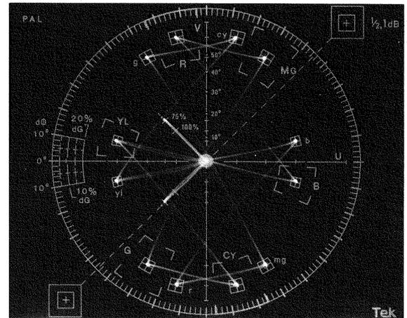
Figure 3. A vectorscope display of Colour Bars.
