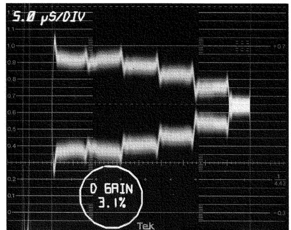
Figure 77. The 1781R double trace DIFF GAIN display showing results. (Attenuation only; peak and peak-to-peak results are the same.)
