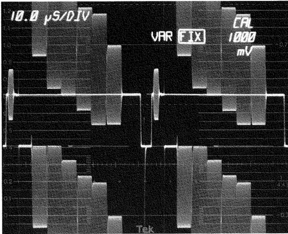
Figure 9. The WFM + CAL mode in the 1781R indicates that insertion gain is properly adjusted.
