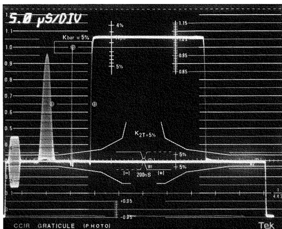
Figure 60. With the pulse taken as the reference, the 1781R graticule indicates that this signal has a  $K_{\text{pulse/bar}}$  distortion of 2%.
