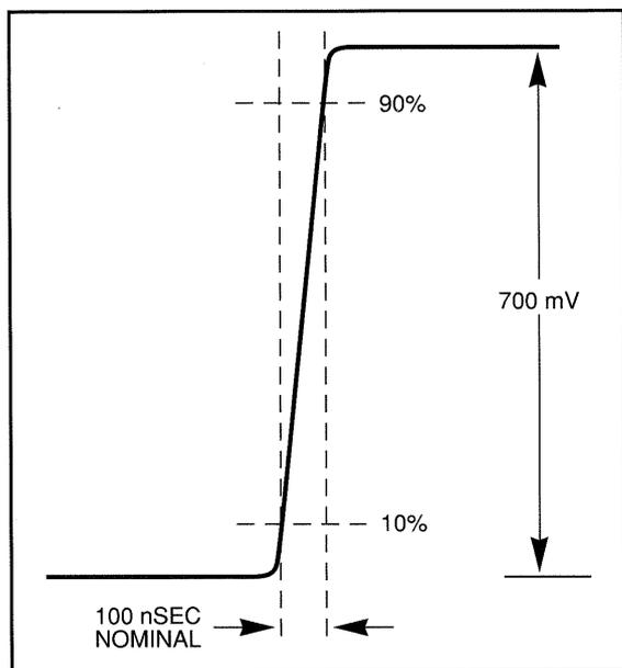
Figure 28. A T rise time bar has a 10% to 90% rise time of nominally 100 nanoseconds.
