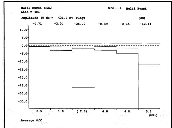
Figure 49. VM700A Multiburst measurement.
