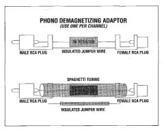
have a moving coil type cartridge with a transformer, <u>DO NOT LEAVE THE TRANS-</u> <u>FORMER IN LINE</u>, as this could potentially damage the transformer and the cartridge. After demagnetizing, remove the adaptor and re-plug the turntable into the phono input. <u>MAKE SURE YOU CAREFULLY TIME TRACK 6.</u> Do not play beyond 0:55. At end of Track 6, stop disc before proceeding to Track 7.
