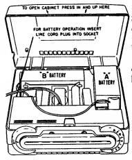
Disconnect the &C line cord from the wall outlet. Squeeze the handle support springs together near the escutcheon to remove the plastic handle. Remove the two escutcheon mounting screws. Remove the "Off-Volume" and "Tuning" knobs. Now open the cabinet (see illustration at left). Loosen the speaker mounting clips, rotate them away from the speaker, and carefully lift the chassis and batteries out of the cabinet.
