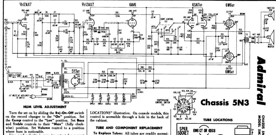
Line cord polarity is very important for correct amplifier operation. If touching the centerpost on the record changer increases the hum level, reverse the line cord in the wall outlet. Touch the centerpost again. Leave the line cord plug in the position that gives the least amount of hum when the centerpost is touched.
