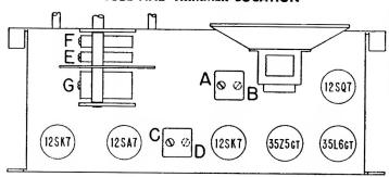
Adjustments B and D are made from underside of chassis.
