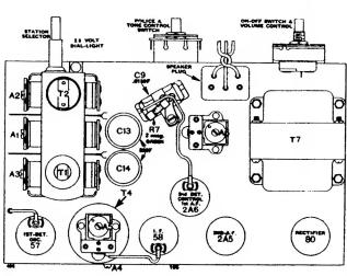
In a few early 165 sets, the tracking condenser C3 is 680MMF. In late sets, C1 is 25MMF instead of 50MMF.
