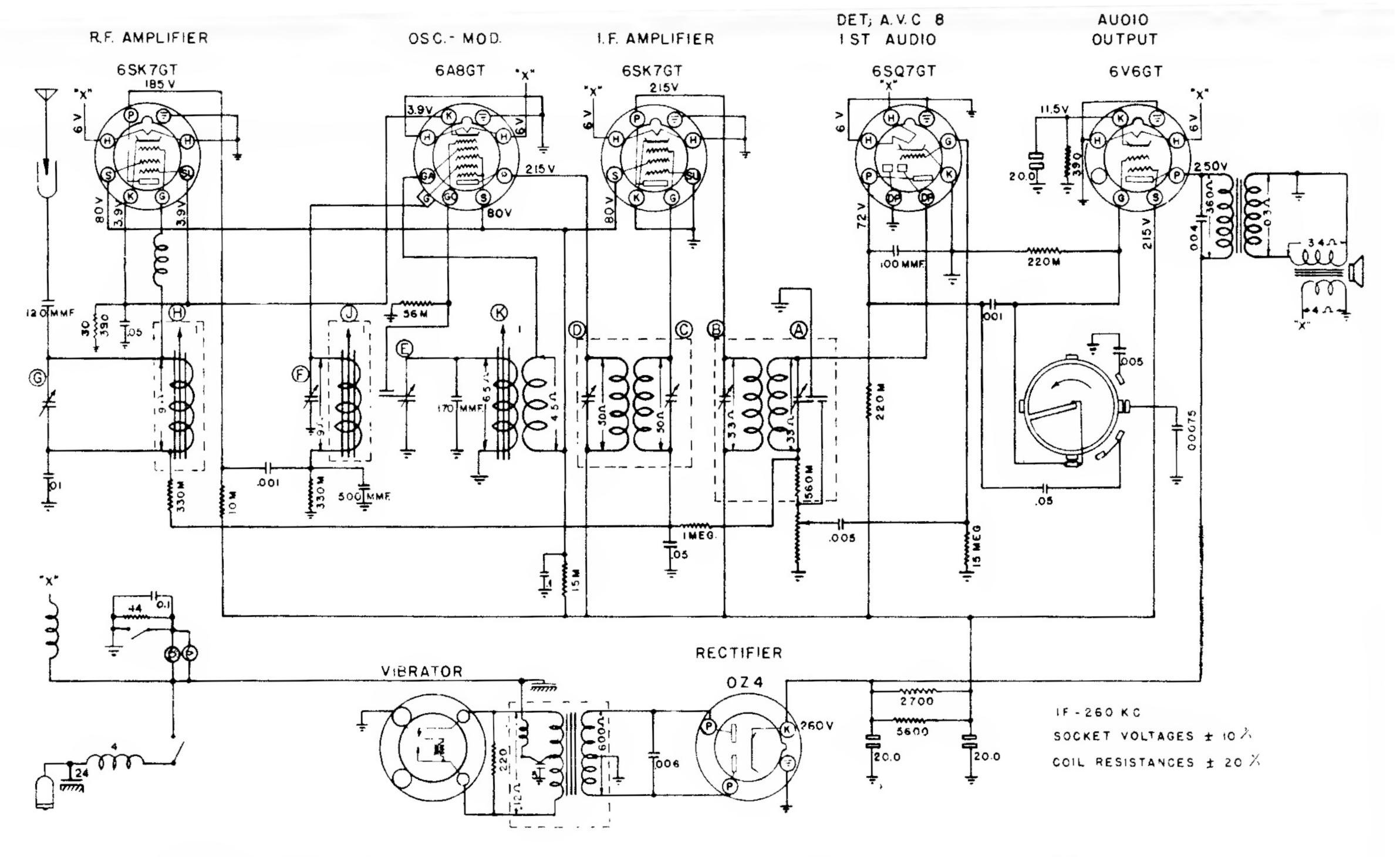
ANTENNA CIRCUIT: The antenna circuit is directly coupled to the antenna. The antenna coil is tuned by means of an iron core and the circuit is adjusted for slight variations in antenna capacity by means of an antenna trimmer located on the bottom of the receiver case.
