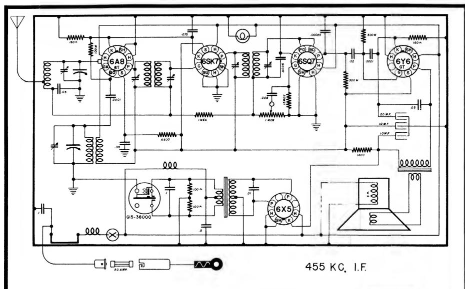
WIRING DIAGRAM—MODEL A-559
