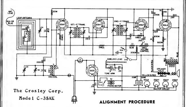
The chassis of this receiver is connected to one side of the power supply and for this reason all test equipment should be thoroughly insulated in order that the power supply will not become short circuited while aligning the receiver.
