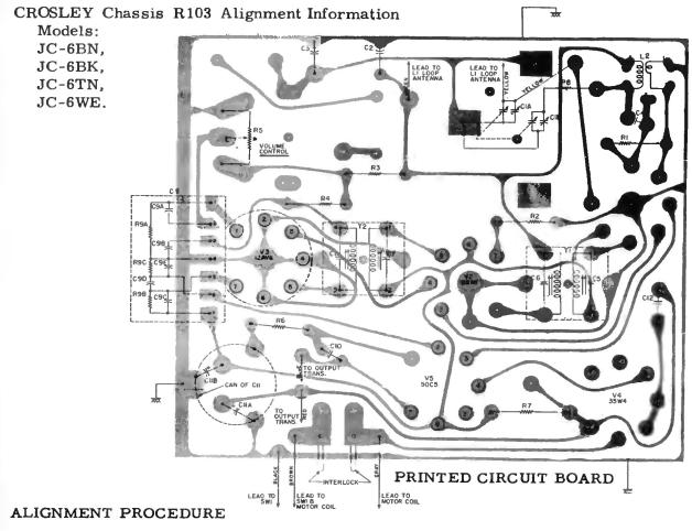
To operate set when it is removed from cabinet, connect switch leads (brown and black leads) together.
