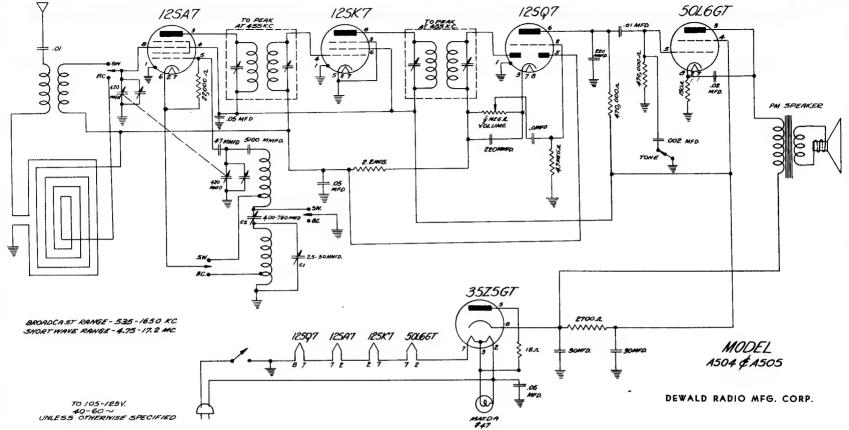
The models A-504 and A-505 are superheterodyns receivers with full automatic volume control. A Loop-tenna is incorporated which makes the use of an antenna unnecessery, in most localities, for broadcast reception. These receivers will function from 105-125 volts, 40-60 cycles A.C. or D.C. power supply. A renge of 535-1650 kilocycles and 4.75-17.2 megecycles, [17½-63H) is covered by these receivers.
