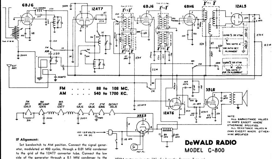
For FM alignment set bandswitch to FM position and leave generator connected to the grid of the 12AT7 converter tube. Adjust generator to 10.7 MC. Connect 20,000 ohm per volt or
