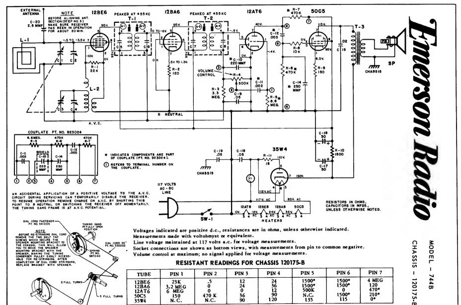
\* Resistances measured to pin 7 of rectifier 35W4 (B+).
