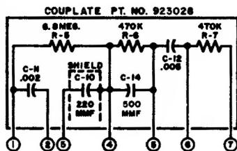
\* INDICATES COMPONENTS ARE PART OF COUPLATE (PART NO. 923026)
