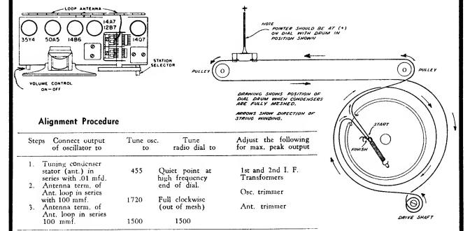
Output meter is connected across voice coil. Receiver volume is turned to maximum.
