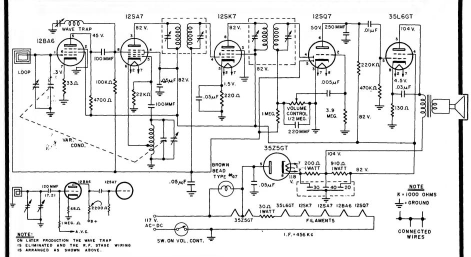
Power supply (40-60 cycles AC) 105-125V AC-DC Power consumption 30 Watts Frequency Range 1680-528 KC I.F. Circuits 456 KC
