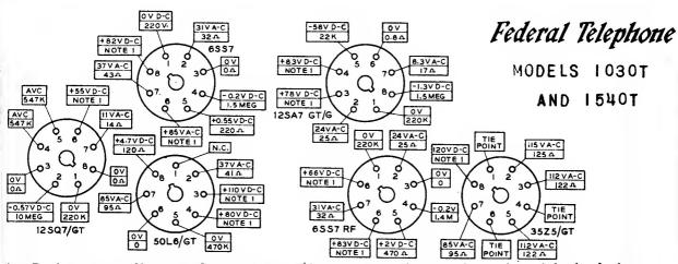
Resistance readings at these points will vary since they are in series with the leakage of the electrolytic condensers which is subject to change.
