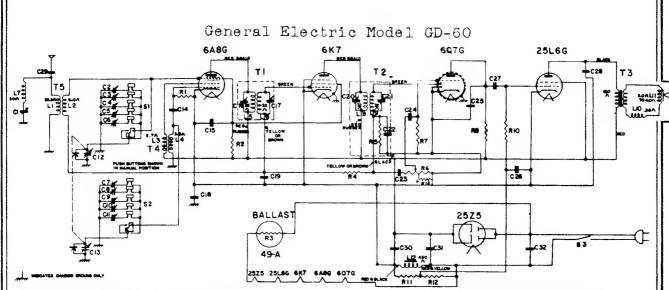
\* Used on early production receivers only. For replacement purposes, use specified volume control and omit R-13
