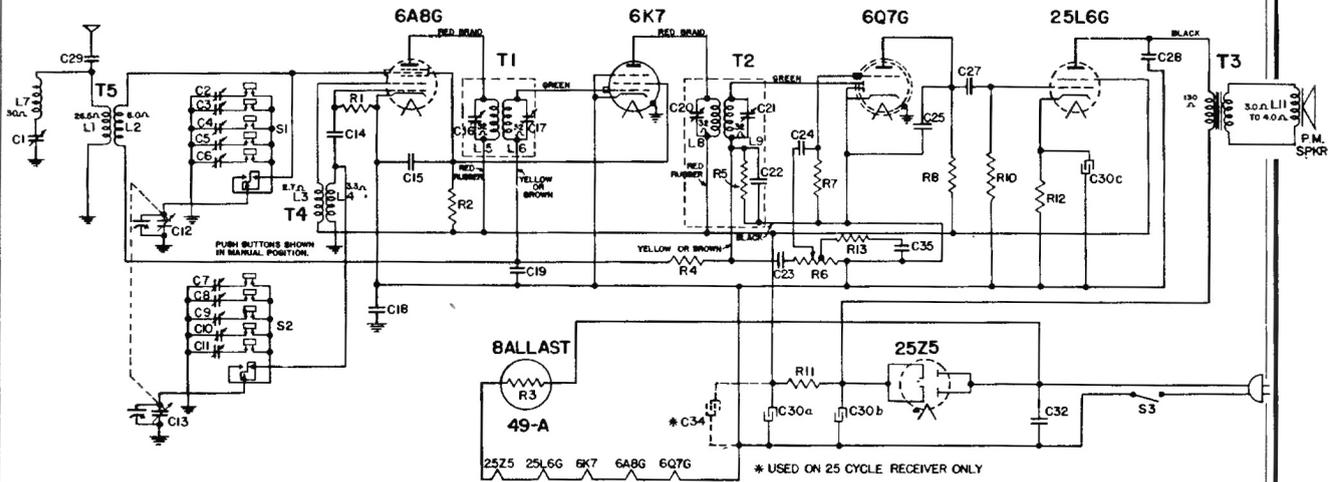
Set test oscillator to 455 and apply signal to the control grid of the 6A8G tube through a .05 mfd. capacitor. Do not remove the grid lead from the 6A8G. Keep the test oscillator output as low as possible to give a readable output. Adjust all four I.F. trimmers for maximum output.
